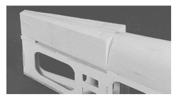
1. Locate the dummy fin and fillet parts on sheet 9. Laminate each with thick CA glue. Find the two large balsa blocks and trace the outline of the dummy fin on the surface of each and saw out. This will give you the profile required. Tack glue the parts together with the dummy fin in the center. Align the block on the **centerline** of the fuselage and mark the fuselage configuration on the bottom side. Saw to shape and tack glue on fuselage.
