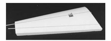
4. Locate the 8 - ¼" sq. hardwood spars and glue them in the spar slots with epoxy or white glue. Make sure they are seated in the groove and flush with the top surface. If groove is too deep apply Balsa Magic on top of spar to make it flush with foam. It is easily sanded after it cures. We cannot control the tolerance on the hardwood strips. Work with the core in the packing to prevent warping.
