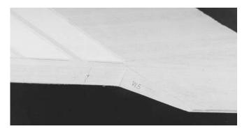
13. Locate W5 and glue in place on the aileron inset inboard end. Cap trailing edge of wing with a  $3/8" \times 1-1/8" \times 36"$  balsa stick. Use white glue and tape in place. Plane and sand top, bottom, and tip end flush with surfaces. Locate hinge hole centers from the aileron. Note: be careful when planing and sanding the wing trailing edge. You have little surface to work with and it is very easy to damage the capping.
