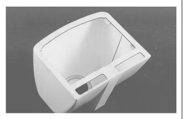
vent holes will make it easier to align. Lay the cowl on its side on a flat surface. Find CW4 and spread some thick CA on one side. Center it over the seam, inside, between the top and bottom cowl halves and against the cowl ring. Now, do the other side.
