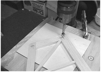
4. Locate the tail bracing hard points from the plans and drill a 3/8" hole, two places, with a Forstner drill bit. Use a backing to ensure a clean break through of the hole.
