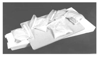
8. Check the packing and core for alignment and place a heavy board on it to distribute the weight. Onegallon plastic zip bags, doubled, filled with sand make excellent weights. Allow to cure over night before removing.
