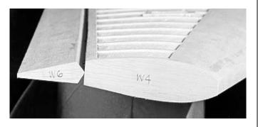
14. Glue on W4 with white glue and tape in place. Sand flush with mating surfaces. Plane and sand the leading edge to the configuration shown on the plans.
