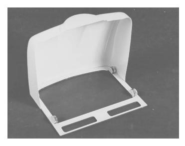
4. Place the cowl ring assy. on a flat surface with wax
