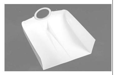
5. Glue in the cowl ring, CW5, with thick CA glue on the lower half cowl.
