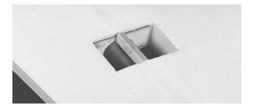
5. Find W3 and W3A and epoxy them on the forward edge of the spar and against the tube in the square cut out area. W3A, on the bottom, has a slight taper so trial fit it first before gluing in.
