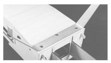
1. Layout the holes to mount the landing gear noting the dimensions shown on the plans. Holes for the wheel pants retaining bolts will also have to be drilled. Locate these holes  $\frac{3}{4}$ " from the axle hole on the centerline. Use a #28 drill to drill one hole in each strut.
