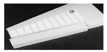
10. Trim and sand the leading edge sheeting flush with the foam core. Locate and install the 3/8° x 1-3/8° x 48° leading edge. Use white glue and masking tape to hold it in place.
