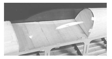
10. Locate the canopy and cut the ends out of it. **Do not remove more than the end pieces.** Mount the canopy base and tape it in place. Lay the canopy over the base and align. Now tape in place. Mark around the periphery of the base with a felt tip pen.. Remove and trim off the excess. Re-mount the canopy. Of course it don't fit. Keep trimming until it does.
