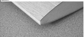
10. When dry, remove the wing from the shucks and sand all the sheeting flush to the wing cores, make sure you keep the center and outboard edges at 90 degrees.
