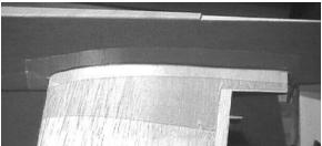
86. Reinforce the tail joint on top and bottom with fiberglass and ca.
