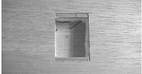
13. Measure carefully, and using the laser cut servo plates as a guide, trim the lower sheeting for the servo hole. It's best to start small, then adjust the hole bigger to fit the plate.
