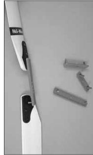
Your Heli-Max Blade Balancer includes (4) different sizes of blade mounting plates and a nylon mounting bolt. Select the mounting plate that best fits the holes in the blade grips. Secure the mounting plate and two blades to the balancer with the nylon mounting bolt.
