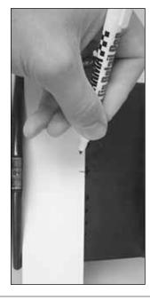
The first step for balancing is finding the center of gravity of the two blades. Place one blade onto the balancer with the leading edge against the side with the level. Shift the blade on the balancer until the bubble indicates level. The middle of the black balancing tray is now at the C.G. of this blade. Mark this position on the blade with a felt tip pen.
