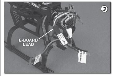
3. Plug the E-Board connecter that was unplugged in Step 1 into the LPM, making sure that the E-Board connector wire colors match the label on the LPM (LPM "-" to Black, LPM "+" to Red, LPM "-" to White).
