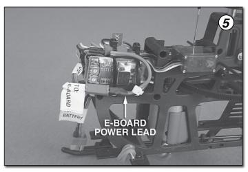
5. Connect the LPM lead labeled "To E-Board" to the E-Board power lead. Use a tie strap to attach the E-Board power lead as shown. Remove the excess tie strap using diagonal cutters or scissors.
