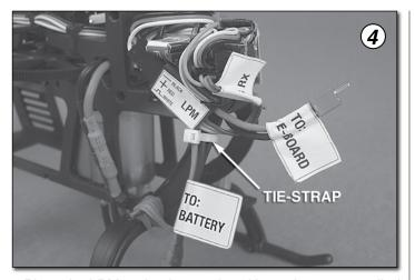
4. Place the LPM under the receiver. Use a tie strap supplied to secure the "To Battery" lead from the LPM to the main frame as shown. Cut the excess tie strap using a pair of diagonal cutters or scissors.
