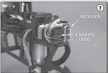
1. Unplug the E-Board lead connector located in the 3rd slot down from the top of the receiver.
