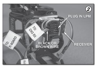
2. Plug the LPM lead labeled "To CH3 RX" into the 3rd slot down from the top of the receiver. The black or brown wire on this connector must be toward the front of the helicopter.
