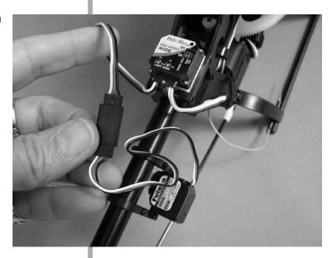
Attach the 3 wire male connector (rudder) from the gyro to channel 4 of your receiver (Futaba®). Also, plug the one wire plug from the gyro (gain) into channel 5 (Futaba), making sure the yellow wire is aligned with the white wire (signal) of the other servo plugs.
