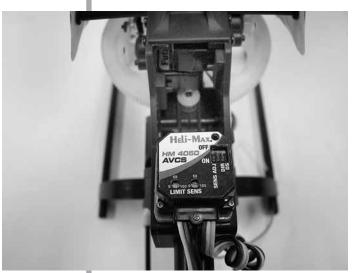
Attach your rudder servo connector to the open female connector leading from the gyro.
