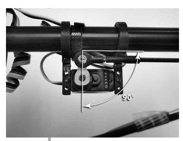
Attach the pushrod to the servo. Then, check the servo direction; simply place the transmitter near the back of the helicopter. Move the rudder stick slowly back and forth. The trailing edge of the tail blades should move the same direction as the rudder stick. If not, use the servo reverse option located on or in your transmitter.
