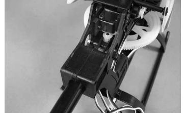
The orientation of the gyro's sensor is such that the label of the gyro faces up. Clean the area with an alcohol pad and attach the gyro using the supplied foam tape. Press down firmly to secure the gyro. To be consistent mount the gyro so the face plate wording is legible from the back of the helicopter.
