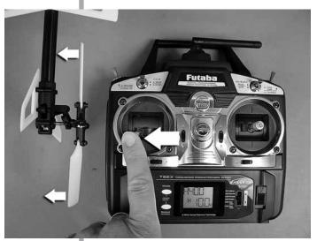
Next, pivot the tail blades so both blades are pointing up. Adjust the length of the rudder pushrod so the distance between the blade tips is 18 to 20mm. Also double check that the pitch slider is centered on the tail shaft. Note: If the rudder servo mounts to the tail boom (Typical), loosening the clamp screws and sliding the servo forward or back on the boom achieves the same adjustment.
