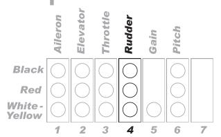
Adjust the trim switch (located under the rudder stick) to the centered or zeroed position. Also, if you have a computer radio, enter the radio's sub trim menu and make sure channel 4 is zeroed.
