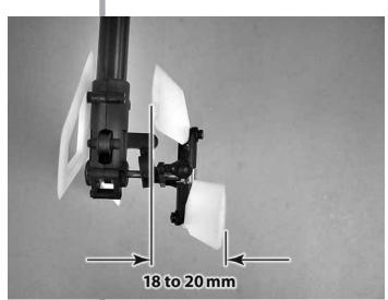
Check the mechanical limits by moving the rudder stick all the way to the right and then all the way to the left. Adjust end points (left and right) using your transmitter's...
