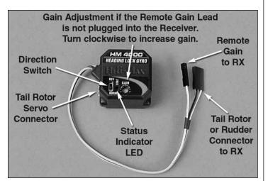
EPA / ATV (Tail Rotor): 70% (Left) / 70% (Right) Dual Rate: 100% (Left) / 100% (Right) Exponential: -40% (Left) / -40% (Right) Trim Step (Tail Rotor Trim): set to 1 after initial flight Gain: Normal 45% (AVCS), Idleup1 45% (AVCS), and Idleup2 45% (AVCS)
