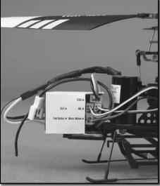
☐ Place a piece of double sided tape on the back side of the ESC (Electronic Speed Control). Mount the ESC onto the E-Board as shown in the picture. Route the ESC lead to the receiver and plug it into the port labeled ESC on the E-Board. It is best to route the wires as shown above and place the E-Board power connector on top of the E-Board to avoid accidental use. Route the ESC power lead out the bottom of the helicopter as shown (the power connector on the E-Board is no longer used).
