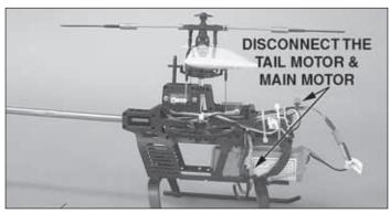
□ 1. Once you are certain the main motor and tail motor are disconnected, turn the transmitter on, center all trims, place the throttle at the 50% position and flip the Idle Up switch to the "ON" position. Plug the flight battery into the E-Board and allow the gyro 10 seconds to initialize. Hold the flybar level and the blades should be
