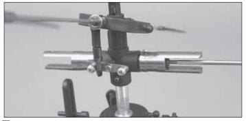
**7**. Place the remaining blade grip onto the spindle. Apply threadlocking compound to the 2mm spindle bolt and re-install into the spindle.
