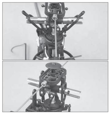
□ 10. Slide the oval links over the blade grips and re-install them onto the flybar control arm and the swashplate.
