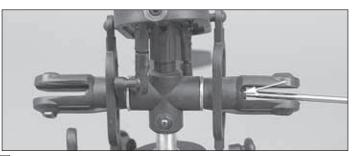
□ 3. Remove the spindle bolt using a 1.5mm allen wrench.
