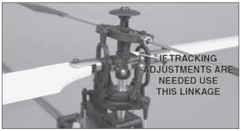
The Axe CP is now ready to fly. Perform the tracking test as mentioned in the AXE CP instruction manual and if an adjustment is needed use the linkage shown above.
