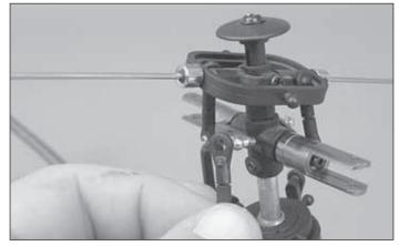
□ 9. Install the control linkage between the blade grip mixer arm inner ball and the swashplate.
