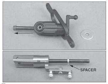
□ 5. Slide the spindle out of the blade grip and insert the spindle into the new Bell Hiller blade grip. Slide a thin dampening spacer onto the spindle.
