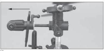
↓ 4. Remove the blade grip from the side you removed the spindle screw from. Pull the other blade grip and spindle out of the head block.
