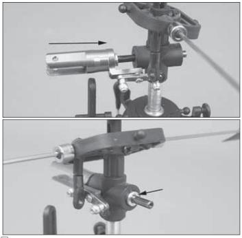
6. Using a 1.5mm allen key, push the new blade grip and spindle through the dampeners. Install the other thin dampening spacer onto the spindle as shown.
