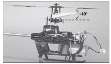
$\Box$  3. Lower the collective stick to the bottom position. You should have -10° of pitch.
