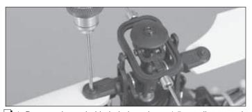
□ 1. Remove the main blade bolts using a 1.5mm allen wrench. Remove both main rotor blades from the helicopter. Remove the 2mm nut from the bottom of the blade grips. These will be needed later when reinstalling main rotor blades.
