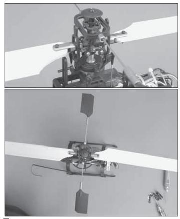
□ 12. Remove a paddle from the flybar. Install one brass paddle weight onto the flybar and re-install the flybar paddle. Repeat on the opposite side. Slide the paddle weights against the paddles and tighten the set screws against the flybar. Measure and verify both paddles are the same distance out from the flybar control arm. Both paddles must be parallel with the swashplate. If you feel the paddles rotate too easily, add a drop of CA to the threads before threading the paddles on.
