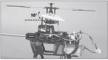
□ 2. Raise the throttle to the uppermost position and you should have 10° of top end pitch.
