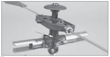
**8**. Remove all of the control links from the rotor head. Verify the new linkages are the same length and have a 1mm gap between the ball links. Please note there is a dimple on one side of the ball link. The dimple must be on the outside as you snap the linkage onto the ball. Install the new control linkage between the flybar seesaw and the blade grip mixer arm as shown above. Repeat this for the opposite blade grip.
