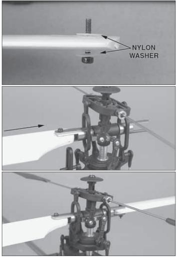
□ 11. Slide one thin nylon washer onto the 2mm main blade screw. Slide the screw with washer through the blade grip and place one thin nylon washer onto the opposite side. Carefully slide the blade and washers into the blade grip. Apply threadlocking compound to the blade bolt and install it using the 2mm nut removed from the blade grip earlier. Repeat for the opposite blade grip.
