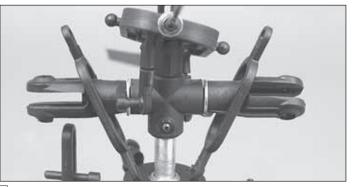
□ 2. Remove the oval linkages from the swashplate and flybar control arm.
