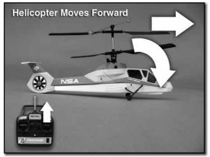
Moving the cyclic stick forward (away from you) will cause the helicopter to tilt forward and start moving that direction.
