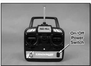
☐ Turn on the transmitter using the power switch as shown and verify that the LED indicator glows solid red. Turn the transmitter off for now. If the LED indicator did not light then remove the battery box and verify that the polarity of the batteries is correct.
