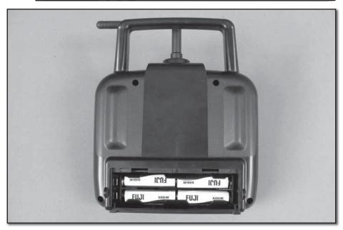
☐ Open the battery cover on the back of the transmitter, and install **four** AA batteries. Double check the polarity of each battery before replacing the battery cover.
