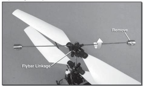
Remove the flybar linkage from the blade grip. Press outward on one side of the head block and simply rotate the flybar carrier from the head block. Once the flybar carrier has been removed, remove the flybar weight bolts and remove the flybar weights. Remove the flybar linkage from the old flybar and install the linkage onto the new flybar. Install the flybar weights onto the new flybar and slide the flybar pivot back onto the head block. Reinstall the flybar linkage.
