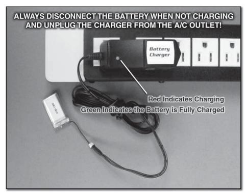
☐ Plug the battery into the charger. The charge indicator light will turn red; this indicates that the battery is being charged. Once the battery is completely charged, the charge indicator light will turn solid green. Disconnect the battery from the charger. Under normal operating conditions, the battery may take up to one hour to recharge.
