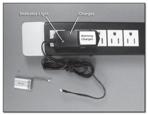
☐ Plug the charger into an AC outlet. The *indicator light* on the wall transformer will flash red during initialization and then turn solid green once initialization has been completed.
