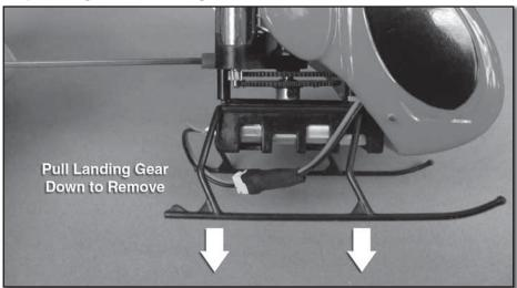
Remove the flight battery and simply pull down on the landing skid. Press the new landing skid into place.
