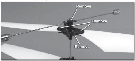
Remove both blade bolts and main rotor blades. Remove the two grip bolts and remove the blade grips. Place the new grips onto the pins. Install the grip bolts and install the blades.
