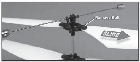
Remove the blade bolt using a #00 phillips screwdriver. After the blade bolt has been removed, slide the rotor blade out of the blade grip. Reinstall the new blade, ensuring that the holes within the blade and blade grip are aligned properly. Reinstall the blade bolt.
