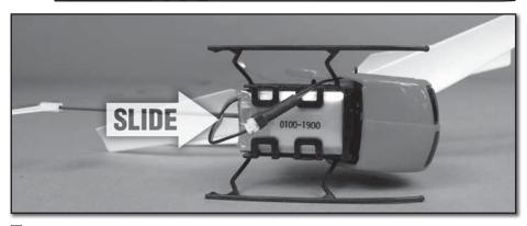
Place the helicopter on its side and slide the battery into the battery compartment. Connect the flight battery and place the helicopter onto a flat surface.
