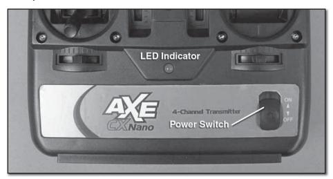
Turn on the transmitter and verify that the LED indicator glows solid red. Turn the transmitter off for now. If the LED indicator did not come on, remove the battery box from the transmitter and verify that the batteries were installed correctly.
