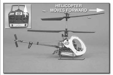
Moving the cyclic stick forward (away from you) will cause the helicopter to tilt forward and start moving that direction.
