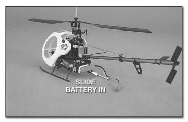
Slide the battery into the AXE CX Micro as shown in the photo above.
