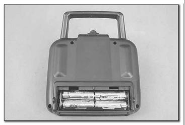
☐ Remove the battery cover from the back of the transmitter, remove the battery box and install eight (8) "AA" batteries into the battery box. Double-check the polarity of each battery before placing the battery box back into the transmitter and replacing the battery cover.
