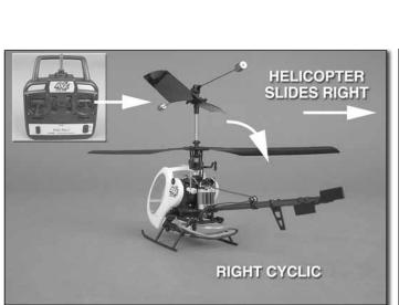
Moving the cyclic stick right will cause the helicopter to tilt right and it will start moving that direction.
