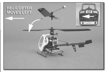
Moving the cyclic stick left will cause the helicopter to tilt left and start moving in that direction.
