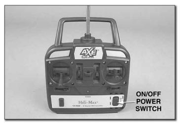
☐ Turn on the transmitter using the power switch as shown above and verify that the LED indicator glows solid red. Turn
