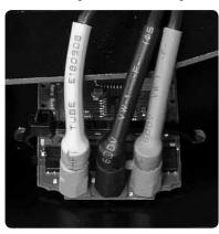
If parts have been replaced, check the motor wires on each ESC. The color of the wire should match the colors on the socket for the front right and rear left ESC.
