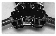
The Voltage 500 3D does not need any assembly. All the non-adjustable bolts have been set to the proper torque and have thread locking compound applied to keep them secure. The tension of bolts that clamp the booms should be checked before each flight by twisting each motor mount. If the boom is not tight, these bolts should be tightened.
