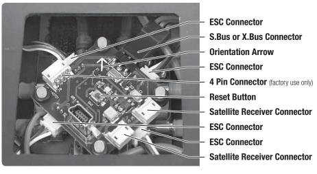
The Flight Controller (FC) has an orientation arrow that must point towards the front of the Voltage 500 3D.
