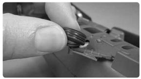
To change the tires grasp the gear leg in one hand and peel away the scale rubber tire.
