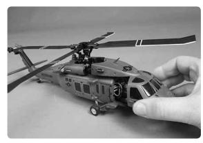
Slide the front portion of the canopy forward to expose the battery compartment.
