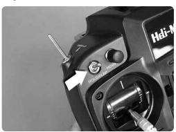
The Throttle Hold Switch (HOLD/FLAP) is used to disable the power output of the motor but has no effect on the other controls. The throttle hold function is intended for autorotation landings off power descent to landing; this maneuver is really not all that realistic in a model this size. In addition to autorotation the throttle hold function can be used as a safety switch while handling the model
