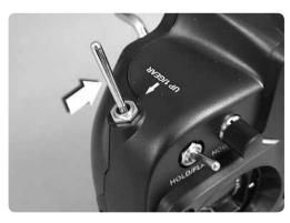
The UP-1 function is enabled and ready to use. The UP-1 Switch (UP-1/GEAR) function is used for aerobatics. If you are a beginner to aerobatics, remember this switch sets the motor speed (see your TX610 manual for details) while still allowing positive and negative pitch control. This means if you get confused flying, pulling the throttle stick back WILL NOT decrease the power to the motor but rather add
