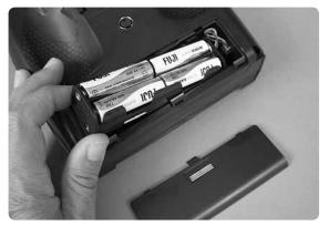
Remove the battery cover from the back of the transmitter and install eight "AA" batteries into the transmitter. Double-check the polarity of each battery before replacing the battery cover.
