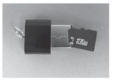
On the bottom of the USB plug is a small notch. There is a slot below the notch where the microSD card should be installed.
