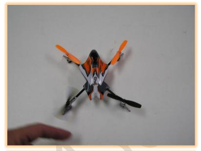
2: Push up on the bottom of the motor to make sure the motor is fully seated upward in the mount. In the event of a crash the motor can shift downward in the mount, pinching the propeller against the motor mount.
