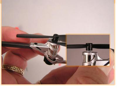
4: Remove the little red rubber cap from the bottom of the motor. You can pry the cap off with your fingernail or hobby knife. Using your included screwdriver, insert it into the hole and lightly push. When done remember to replace the rubber cap! In some cases the impact can be severe enough to shift the motor end bell. This step helps re-seat the part.
