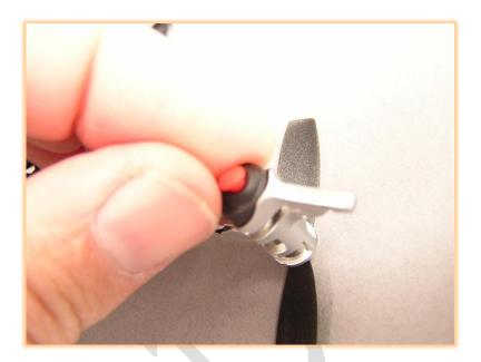
5: Re-spin the prop as you did in the beginning. It should spin freely. It's also a good idea to check to see if you might have bent a motor shaft; having said this, the propeller should spin straight and true.
