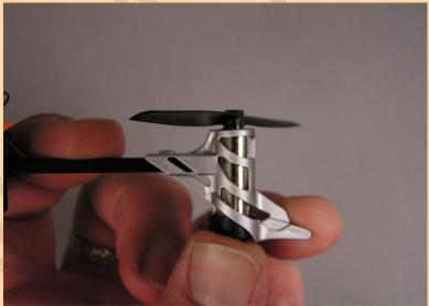
3: The propeller can slide down the shaft pinching the propeller against the motor can. After following step two it's best to check the clearance of the parts. We have found that the best distance between the prop and the motor mount is about 1mm, or the width of a hobby blade. You can use your hobby knife to pry the blade away from the motor mount if needed.
