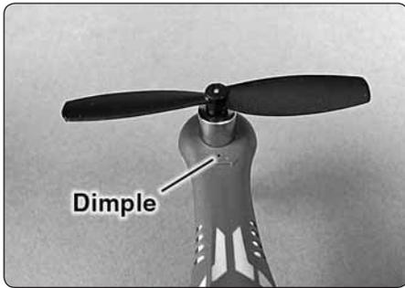
☐ Slide the guard over the motor and position the hole for the mounting screw over the dimple on the top of the arm.
