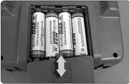
❑ Install 4 AA batteries in the transmitter by removing the battery cover from the back of the transmitter. Double-check the polarity of each battery before replacing the battery cover.
