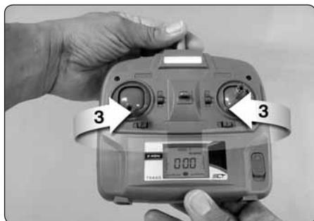
Hold the transmitter by the antenna and bottom with antenna pointed away from you. Rotate the transmitter left to right three times. Rotate it three more times from right to left.
