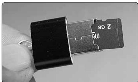
Install the MicroSD card into the reader. Plug the reader into the USB port of your computer.
