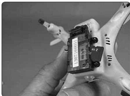
Remove the SD card from the protective case. Flip the model over and push the SD card into the slot on the side of the camera module. When the card is correctly installed, it will click. To remove the card, simply press on the card again and the inner spring system will help eject the card. Note: The card must be in place to capture video or Pictures. The camera has no internal memory.
