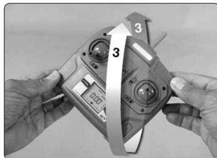
Hold the transmitter by the upper right corner and lower left corner so the antenna is pointed 45 degrees to the right. Rotate the transmitter three times with the antenna moving toward you, then three more times in the opposite direction.
