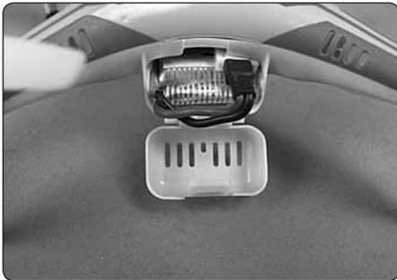
☐ Turn on the TX465 transmitter. Install the flight battery by sliding the battery into the battery compartment. Connect the battery to the power connector and tuck the wires on the side of the compartment. Place the quad on a flat surface and wait for 2 seconds to allow the TAGS-FX control board to calibrate.
