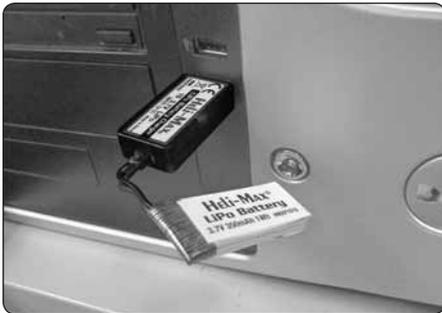
Plug charger into a USB port. A steady red light will glow letting you know the battery is charging. The light will flash slowly when the charge is complete. Remove the battery from the charger. Under normal operating conditions, the battery may take up to 60 minutes to recharge. Never leave the battery attached to the charger after charging is complete.
