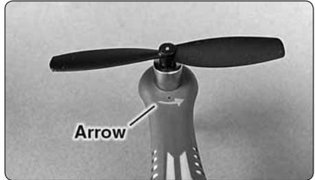
When installing the rotor blades on the 1Si, please use this photo as a guide. There is also an arrow molded on the frame to show the direction the rotor blades will spin.
