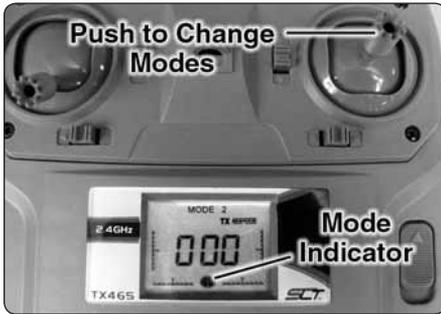
The TX465 transmitter has a dual rate function. This feature toggles between a flight mode that reduces the model's range of motion to make the 1Si easier to fly and one that allows the full range of motion so the 1Si can fly in a more aggressive manner. To toggle between these two flight modes, press down on the right control stick and release it. When the transmitter is in low rates, the ellipse in the lower center of the
