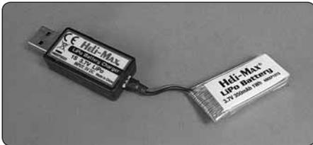
Plug the flight battery into the end of the USB charger.
