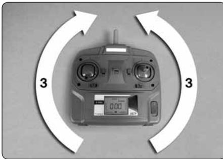
Place the transmitter down on its back with the antenna pointed away from you. Slowly rotate the transmitter clockwise three times, then three times counter-clockwise.
