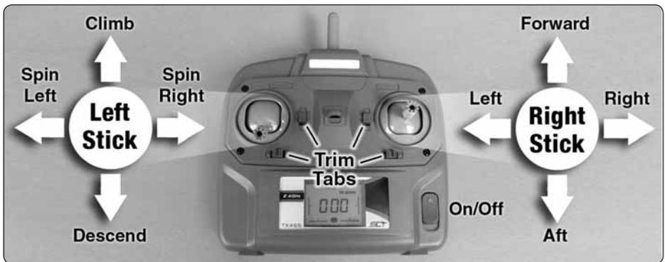
All controls are described with the tail pointing directly toward you. This is the best way to fly in the beginning since it keeps the control inputs oriented the same direction.
