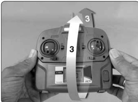
Pick the transmitter up by the sides and rotate it so the antenna moves toward you. Rotate it three times, then three more times in the opposite direction.
