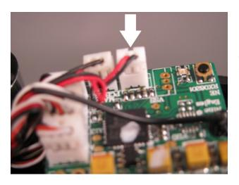
Unplug the LED Gear Contact Board assembly from the E-board and remove the contacts from the model.
