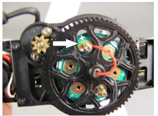
Be sure to connect the red wire that comes up from the main shaft to the post with the "+" symbol. Also, tighten the screws on the posts so they are snug. If these screws are over-tightened, the screws can break the wires.
