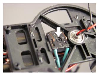
Remove screw that holds the LED Gear Contact Board to the frame.
