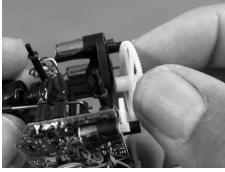
The landing gear will have to be removed to allow access to the main gears. Use the supplied screwdriver to loosen the screws that hold the lower main gear in place and slide it off the inner rotor shaft. The upper main gear can be pulled off the outer rotor shaft without removing any other parts.
