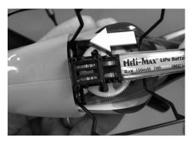
rise. Slowly advance the throttle to test the motors. While the motors are spinning slowly, move the rudder control left and right. The nose of the helicopter should respond by moving the same direction as the left stick. Reduce the throttle after you have verified that all the controls are working properly. Move to a safe distance away from the model when you are ready to take off.
