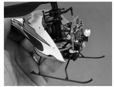
There are two pegs on each side of the fuselage that hold the two sections of the fuselage to the frame. Carefully push the back edges of the canopy outward and slide the rubber grommets off the pegs. Then slide the canopy forward to remove it from the frame. Follow the same procedure to loosen the rear fuselage and pull the frame forward to remove it.
