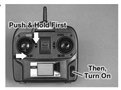
Let go of the trim buttons and you will see 1-1 or 1-0 displayed. The first Digit is the channel number. To change the channel you want to reverse, push down on the right stick. To reverse the travel direction, push the elevator trim button up or down so the second number changes. The V-Cam travel direction settings should be "1" for all channels.
