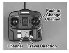
To confirm the change and exit to normal operation, push down on the left stick. The changes will not be saved if the power is turned off before the left stick assembly is pushed down.
