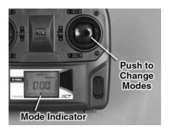
center of the LCD screen will show a half ellipse and emit a single low pitch single beep. For high rates, the ellipse will be complete and the transmitter will emit a single high pitch beep.
