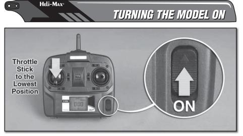
Move the throttle stick to the lowest position and then turn the transmitter on.
