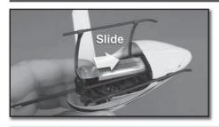
□ Slide the flight battery into the battery compartment. **NOTE:** The battery will only install one way. The helicopter will be "**ON**" at this point.
