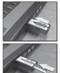
□ Plug the USB charger into your USB port. The *power indicator light* on the charger will illuminate red indicating that the charger is ready for use.
