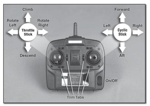
All controls are described with the tail pointing directly toward you. This is the best way to fly in the beginning since it keeps the control inputs oriented the same direction. Once you start getting comfortable you can work on side hovering and nose-in.
