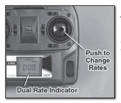
The dual rate switch provides dual control rates for the cyclic and tail rotor controls. Please use the low rate until you become accustomed to your Axe 100 FP. Change the dual rate using a quick push of the right stick. To adjust the dual rate, push and "hold" the right stick and move the throttle stick to the desired percentage. Release the right stick to set.
