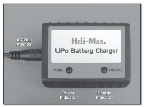
☐ Plug the wall transformer into an AC outlet. The *power indicator light* on the charger will illuminate red and a continuous tone will be emitted indicating that the charger is ready for use.
