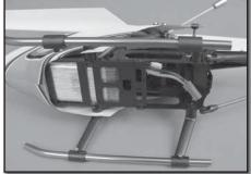
☐ Slide the flight battery into the battery compartment and close the battery door.
