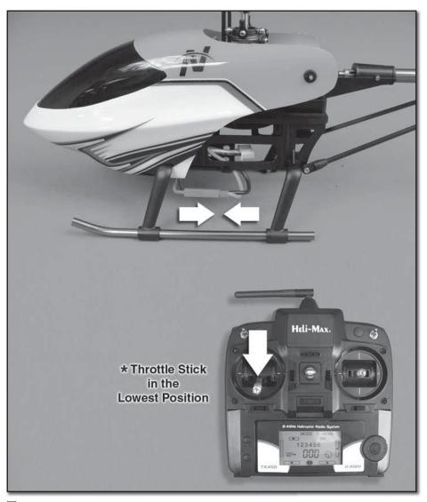
☐ Verify that the throttle is in its lowest position on the transmitter. With the helicopter on its side, connect the battery to the helicopter. Allow the helicopter to remain still for 10 seconds during initialization. After 10 seconds you can place the helicopter on its skids for takeoff.
