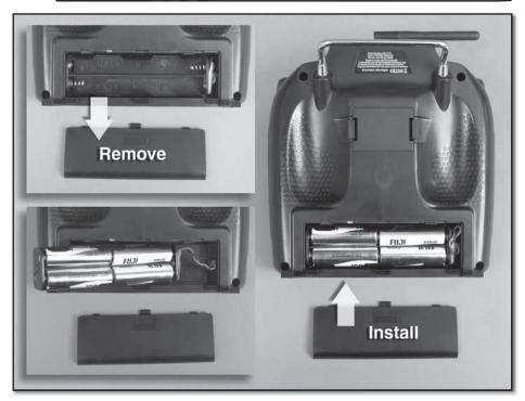
□ To open the battery compartment push inward and pull downward on the battery cover. Carefully remove the battery holder and install eight AA batteries. Double check the polarity of each battery and ensure that the battery holder is connected to the transmitter. Place the battery holder into the transmitter and slide the battery cover back into place.
