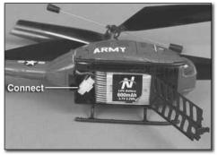
4. Install the Flight Battery and connect to the ESC. Close the battery cover.
