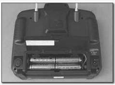
3. Install (8) AA Alkaline batteries into the transmitter.
