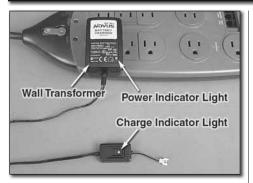
☐ 1. Plug the wall transformer into an AC outlet. The *power indicator light* on the wall transformer will be green and the *charge indicator light* will be solid red.
