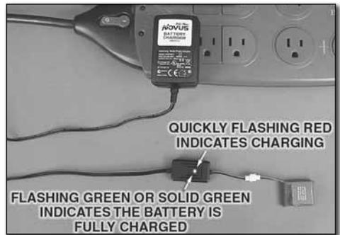
2. Plug the battery into the charger. When the battery is completely charged, the charge indicator light will turn green (solid or flashing). Disconnect the battery from the charger.
