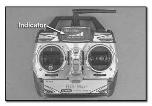
□ Turn on the transmitter using the power switch as shown above and verify that the indicator illuminates. Turn the transmitter off for now. If the indicator did not illuminate, remove the battery box from the transmitter and verify that the batteries were installed correctly.
