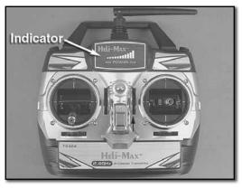
□ The Novus Helicopter uses a 2.4GHz system that requires a binding process when the unit is powered up. This process involves connecting the flight battery to the ESC with the transmitter turned off. Ensure that the throttle stick is at its lowest position and turn the transmitter on. You will notice that the transmitter logo begins to flash, indicating that the binding process is taking place.
