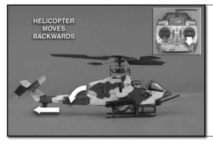
Moving the cyclic stick backwards (towards you) will cause the helicopter to tilt backwards and start moving that direction.
