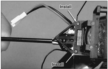
Align the lower tail boom assembly holes with the main frame holes and install the two lower tail boom assembly mounting screws.
