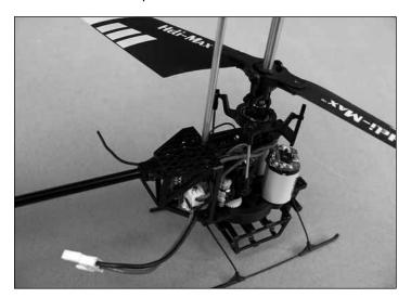
Once you are certain that the holes are lined up properly between the tail boom assembly and the main frame, install the upper tail boom mount screw.
