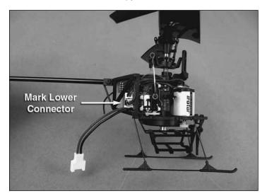
Place a mark on the lower motor connector with a permanent marker. This will help to ensure the connector is placed back into the correct slot during reassembly.
