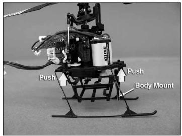
Place the battery holder as shown. Please note that the two body mounting posts must be in front of the drive motors. Push the tabs up through the frame and they will snap into place. After installation, pull downward on the battery tray at each tab position to ensure the tabs have properly engaged the main frame.
