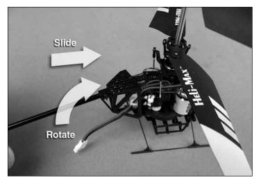
Carefully slide the lead and antenna wire through the tail boom assembly as shown. Place the tail boom assembly back onto the helicopter.
