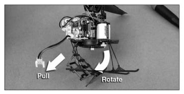
Remove the aft battery tray mounts by rotating the battery tray downward, while pulling the battery tray away from the frame.
