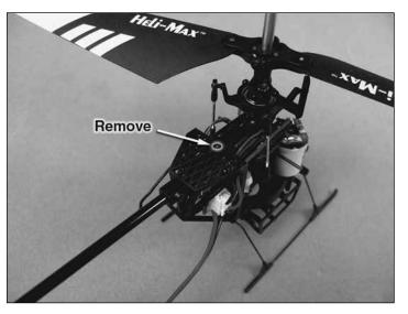
Remove the upper tail boom mount screw.
