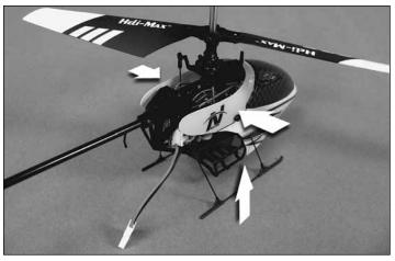
Place the body onto the lower canopy mounts and slide the canopy grommets onto the upper canopy mount.
