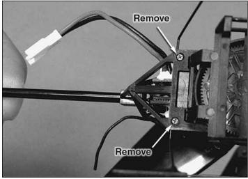
Remove the two lower tail boom mount screws.
