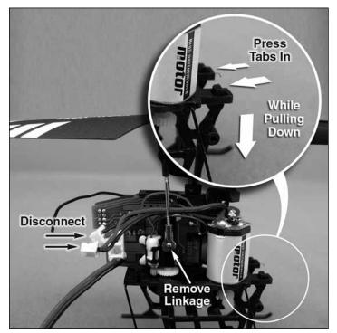
Disconnect the two motor connectors from the 5 'in 1 board. Pull outward on the control linkage to remove it from the servo arm. Repeat this step for the other control linkage. Next, the battery tray must be removed by pressing back on the tabs, using a small screwdriver, while pulling downward on the battery tray.
