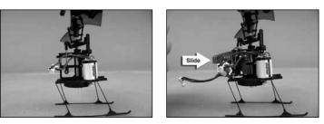
Align the board with the molded channels in the main frame and carefully slide the new 5 'in 1 board into the frame.
