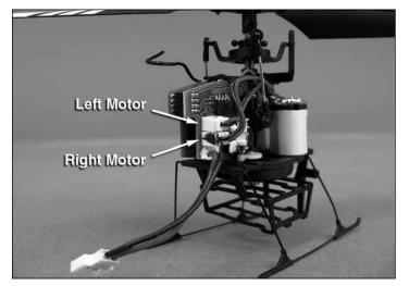
Ensure that the connector you marked earlier is placed into the bottom connector on the board. Reconnect the main motor connectors to the 5 'in 1 control board. Snap the control links back onto the servo arms.
