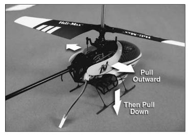
Carefully pull outward and slide the canopy grommets off of the upper canopy mount. Pull the front of the canopy downward (off of the lower canopy mount) and then pull forward, to remove the canopy.
