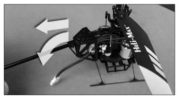
To remove the tail boom assembly, carefully rotate and pull the tail boom assembly away from the mechanics.
