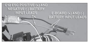
☐ It will be necessary to solder the E-Board and C-12 ESC to the battery connector as shown above. If you decide to use the Great Planes 910mAh LiPo battery (GPMP0815), we suggest installing a Deans Ultra Male Plug onto the ESC and E-Board to match the connector on the battery pack. The Deans Ultra Plug will better handle the increased current draw of more aggressive flight as your skill level advances.
