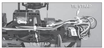
Use two tie straps to attach the gyro wires to the frame. Bundle the wires and ESC together at the front of the helicopter.
