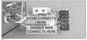
Remove the orange wire from the receiver and plug the GY240 into the same position. Verify the black wire (-) on the connector is towards the outside edge of the receiver. Now plug the orange connector into the next available position on the receiver (channel 5), and align it with the column of white wires on the other connectors.
