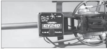
On the gyro, set the "AVCS" switch to "ON" and set the "DIR" switch to "REV". Set the gain to 60% using the adjustment dial on the gyro. If necessary, adjust the gain to match your flying style or desired setup. The typical range of gain is 50% to 75%.
