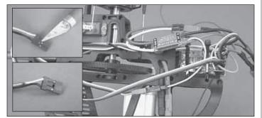
☐ Since the E-Board provides power to the receiver and servos, the BEC in the C-12 ESC must be disabled. Carefully lift up the plastic tab on the C-12 ESC connector, remove the red pin from the plug, and fold it back over the wire. Wrap a piece of electrical tape or heat-shrink tubing around the connector pin and wire. Plug the C-12 ESC into the GY240 gyro.
