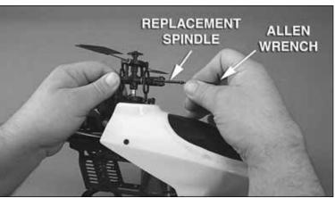
5. Insert the 1.5mm allen wrench into the remaining bolt in the spindle. Insert the replacement spindle into the blade grip where you removed the screw. When performing the next step, hold onto the blade grip on the opposite side of the rotor head. Use the 1.5mm allen wrench to press the replacement spindle through the head which will push the old spindle out the other side. Discard old spindle. Make sure no parts fall out during this step.
