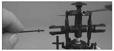
**6**. Install the 2x6mm socket head cap screw and 2mm washer you removed from the replacement spindle earlier using a 1.5mm allen wrench. Tighten the bolts with both 1.5mm allen wrenches.
