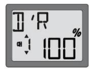
Dual rates on the 6EX-2.4GHz are factory-preset at 100% for Channels 1, 2 and 4. Dual rates on Channels 3, 5 and 6 are not adjustable.
