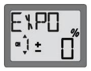
Press the Data Input Lever *down* (-) until the setting for Channel 1 is "-30." Now flip the dual rate switch to the other position and use the same method as above to set the expo "-30" for this rate. This step will assure that there is expo programmed on both rates which could prevent problems if the dual rate switch is inadvertently placed on the wrong position during flight.
