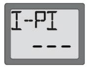
The first screen you'll see is for Point 1. The "%" sign should be blinking. To program each point, press the Data Input Lever up (+) until you reach the required setting. To advance to the screen for the next point, press the "SELECT" key.
