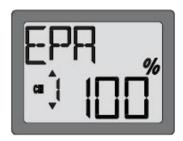
Only Channels 1, 2 and 3 need to be programmed. Channels 4, 5 and 6 should stay at the factory setting (100%).
