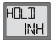
Push the Data Input Lever up (+) to change from "INH" to "ON".
