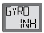
Push the Data Input Lever up (+) to change the screen from "INH" to "ON."
