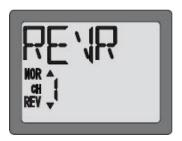
The number "1" will be flashing. This stands for Channel 1. Channels 1 and 2 should already be in "NORMAL" position. The servo on Channel 3, however, should be reversed. To reach Channel 3, press the "SELECT" button twice. Reverse the servo by pressing the Data Input Lever *down* (-) once.
