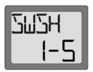
No action required. The 6EX-2.4GHz is factory-set at "1-S". The reading should already be on-screen and blinking.
