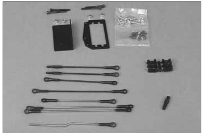
Bag 4 Contents: Tail Rotor Servo Mount, Linkage Rods, Tail Rotor Pushrod Coupler, Servo Retainers
