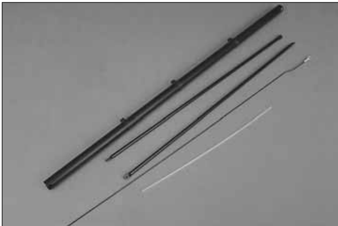
Bag 8 Contents: Tail Boom, Tail Boom Supports, Tail Rotor Pushrod, Antenna Tube
