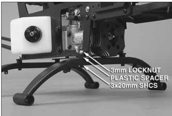
Bag 6 Contents: 3x20mm SHCS (4), Plastic Spacers, 3mm Nylon Lock Nut (4), 3x4mm Set Screws (4)
