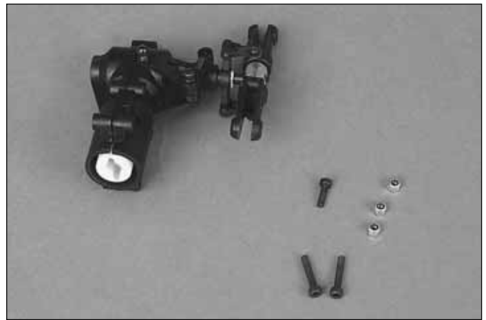
Bag 8-2 Contents: 3x16mm SHCS, 3x10mm SHCS, 3mm Nylon Lock Nuts
