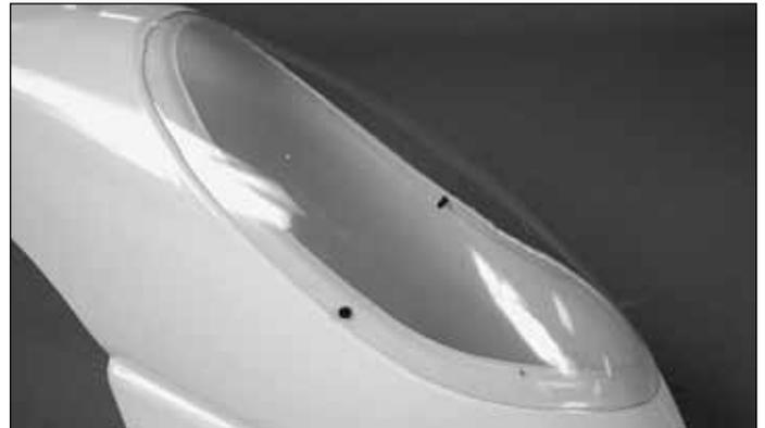
11. Secure the shield to the canopy with the two small screws packaged with the shield.
