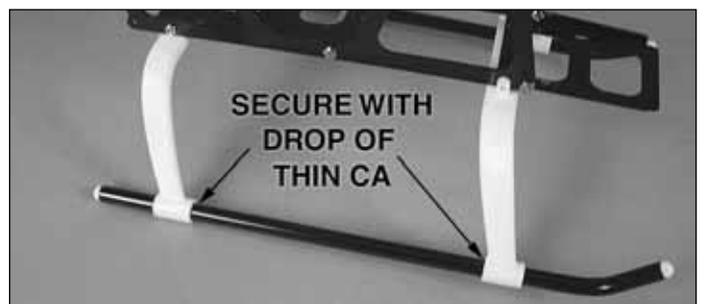
12. Secure the landing gear skids by positioning them correctly and adding a drop of thin CA at each joint.
