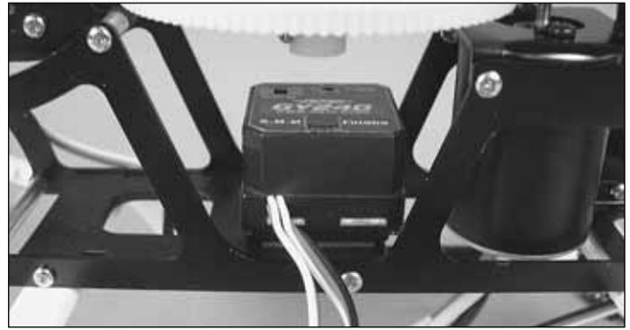
❑ 3. Install the gyro directly under the main shaft. Connect your rudder servo to the gyro's output port.
