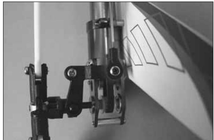
3. Connect the ball link to the ball on the tail rotor pitch control horn. Check to see that the ball link runs freely on the ball, and loosen it if necessary using the following Heli-Max Tip.
