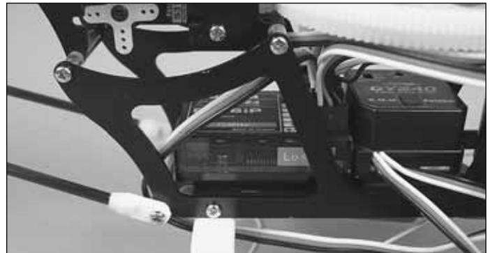
❑ 4. Install the receiver in the position shown. Connect your servos and gyro to the appropriate channels.
