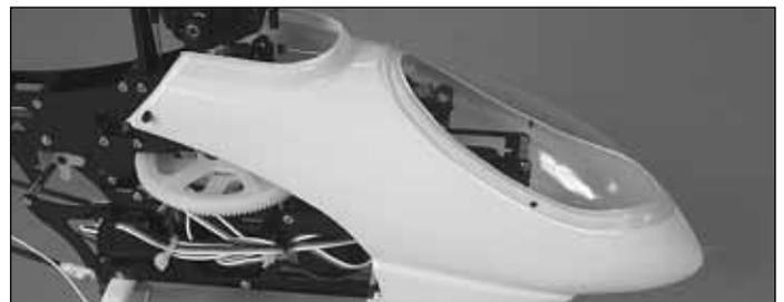
12. Install the canopy onto the helicopter.
