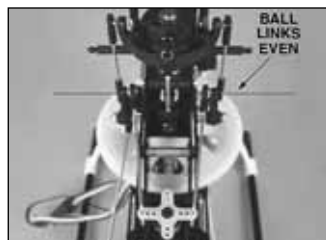
2. Center the aileron servo. Install the aileron pushrods through the servo arm and install the servo arm on the servo as shown. With the servo centered, the two aileron control horns should be even with one another. If they are not, adjust the pushrod until they are. Once you have the aileron control horns even, check to make sure that the
