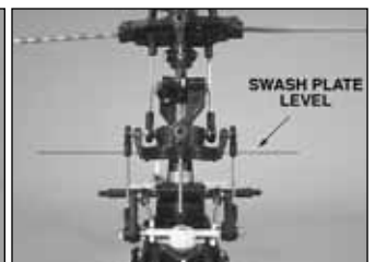
2. Center the aileron servo. Install the aileron pushrods through the servo arm and install the servo arm on the servo as shown. With the servo centered, the two aileron control horns should be even with one another. If they are not, adjust the pushrod until they are. Once you have the aileron control horns even, check to make sure that the
