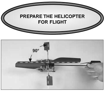
□ 1. Rotate the main blades so that they are pointing away from each other and perpendicular to the flybar. **Note:**
