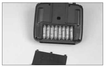
□ 2. Remove the battery cover from the back of the transmitter. Install eight "AA" batteries (not included) in the transmitter. Double-check the direction of each battery before replacing the battery cover.
