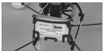
□ 2. Slide the **charged** battery into the battery mount. Secure the battery with a rubber band across the top. DO NOT connect the battery at this time.
