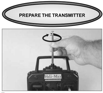
$\Box$  1. Install the transmitter antenna by inserting it into the hole in the top of the transmitter and screwing it into place, using a clockwise rotation.
