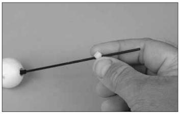
□ 2. Slide a skid mount onto each training gear leg.
