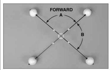
□ 3. Install the gear legs in the center mount. Note that angle A is larger than angle B. The larger angle A faces forward.
