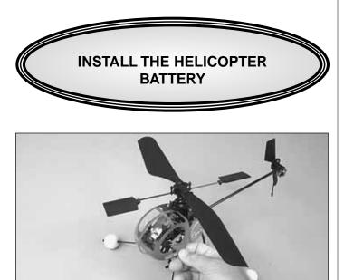
□ 1. Remove the canopy by pulling one side off the horizontal mount, then the other. Note: Be careful to not widen the canopy too much, as it will separate the seam on the bottom of the canopy.
