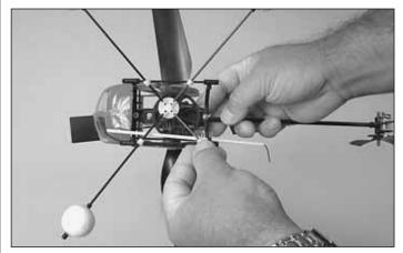
□ 4. Snap the training gear onto the landing gear skids.
