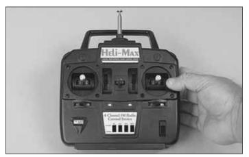
□ 3. Turn on the transmitter and check the LEDs on the front. The green and red lights should be on. If the green light is off and the red light is blinking, new "AA" batteries need to be installed.
