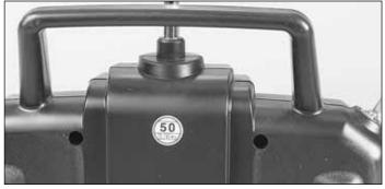
□ 1. Make sure no one is operating any type of R/C equipment on the same frequency as your RotoFly helicopter. The frequency is identified on the back of your transmitter. When you know it's safe, switch the radio transmitter on and fully extend the antenna.
