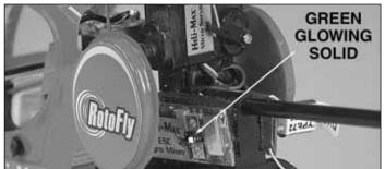
□ 3. Once the plugs are connected, wait ten seconds for the control board and gyro to initialize. DO NOT move the helicopter during this process. During this time, a green light will blink on the control board. When the green light stops blinking and glows solid, your RotoFly is ready for flight. **Note**: If the light does not stop blinking, check that the throttle stick and the throttle trim are both down.
