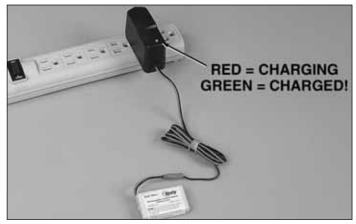
□ 2. Plug the battery into the charger. The light on the charger will turn red. **WARNING:** Do not leave the battery unattended while it is charging. If the battery becomes hot disconnect it immediately.
