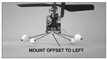
□ 5. Position the training gear so that the center mount is offset to the left of helicopter center. This makes the helicopter lean to the right and helps the helicopter lift off straight.
