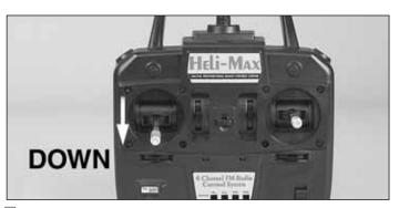
□ 2. Confirm that the left stick is all the way down to make sure the rotor blades do not rotate when the RotoFly's power is turned on. Plug the battery pack into the electronic speed control located on the helicopter.
