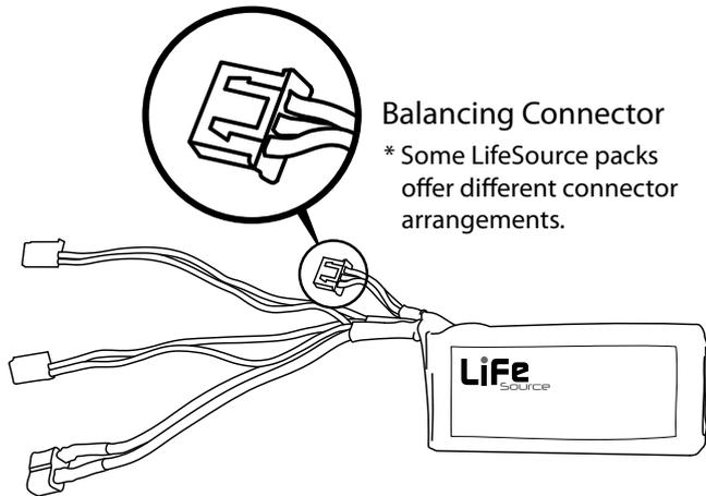
1. Always observe the correct polarity when connecting the battery to the charger and refer to the instructions that came with the charger. For LifeSource batteries having a balancing connector, attach this lead to the balancing port on the charger.
