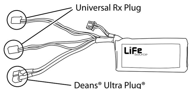
■ A voltage regulator might be required to step the LiFe battery voltage down to an acceptable level when used with some receivers. Check with your radio manufacturer for details. Some servos have a maximum input voltage of 4.8V or 6.0V.
