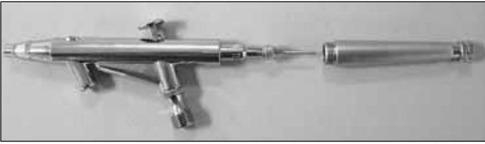
Remove the air hose from the airbrush so that it is easier to work on. Remove the handle from the body of the airbrush.
