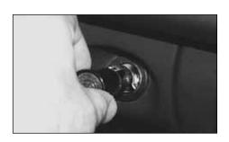
☐ 2. Remove the battery pack from the plane. Plug the battery pack into the charger connector. The battery pack will plug in only one way.
