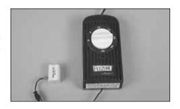
3. Rotate the timer knob on the charger to 20 minutes. Make sure the red light comes on.
