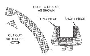
**3**. Cut the cradle sponge into four pieces – two pieces 6-1/2" long and two pieces 3-1/2" long. With a pair of scissors, carefully slit the tubing in a straight line from one end to the other. Cut a 90 degree notch about 3/4 of the way through the diameter of the tube on one end of each of the four pieces. Glue the pieces of cushion to the cradle so that the notch is at the corner. Do not glue the cushion to the bottom of the cradle since the two parts have to slide in relation to each other.
