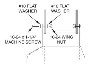
**4.** Each cradle is attached to your field box with a  $10-24 \times 1-1/4$ " machine screw, two #10 flat washers and a 10-24 wing nut.
