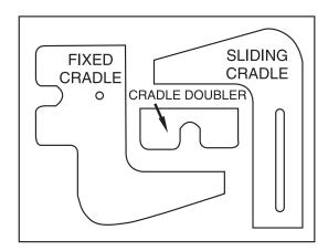
1. Punch out the two, 6 piece sets of cradles and very lightly sand the edges if necessary to remove any splinters. Glue each fixed cradle, cradle doubler and sliding cradle to another piece exactly like it. Make sure they are lined up correctly and that the punched indentation is showing on the largest pieces. You should now have two sets of three different pieces.
