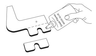
**2**. Glue the cradle doublers to the fixed cradles as shown in the sketch again making sure they are lined up correctly. Drill a 3/16" hole in this assembly where the punch mark is located. Repeat this procedure for the other set.
