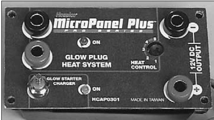
**Congratulations** on your purchase of the MicroPanel Plus™ from Hobbico®! Combining very practical functions in a tiny package makes this power panel an excellent choice for discriminating modelers. MicroPanel Plus is capable of supplying power to 12V field equipment such as starters and fuel pumps, in addition to supplying 1.2V and adjustable heat to glow plugs, and charging 1.2V glow starters with a built-in charging terminal.
