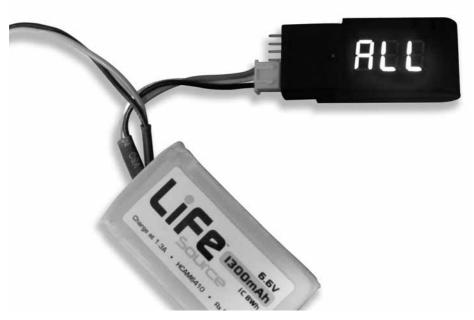
1. For ElectriFly style balance connectors: Simply plug the balance lead from the battery directly to the LVM. The black wire on the balance lead should be connected to the (–) pin on the LVM.
