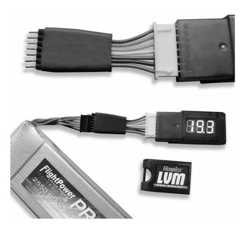
2. For FlightPower/Thunder Power batteries: The included adapter will need to be installed prior to measuring the battery voltage. First connect the adapter to the LVM. Then connect the balance lead from the battery to the LVM.
