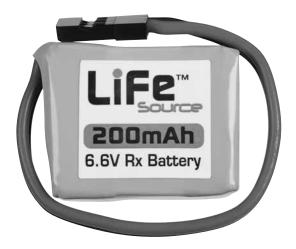
The Life Source 200mAh 6.6V Rx Battery does not have a balance lead for charging. The balance lead has been omitted due to the unlikelihood that the cells would become unbalanced during the 1C discharge (0.2 amps), and to minimize overall weight. Please *do not* charge or discharge the Life Source 200mAh 6.6V Rx Battery above 1C (0.2 amps).
