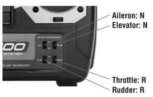
3. Make sure the servo reversing switches on the TTX600 are in the positions shown.
