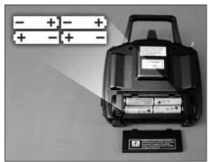
1. Install (4) AA batteries in the TTX-600
