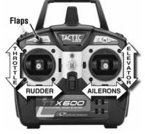
(It is not recommended to exceed 1/3 of the full dial throw on the TTX600 while operating the Cessna 182. Applying more than 1/3 throw could cause excessive flap throw and make the Cessna 182 difficult to control.)
