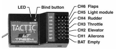
2. Make sure the correct leads are plugged into the TR624 RX in the proper order and that TR624 is secured to the aircraft.
