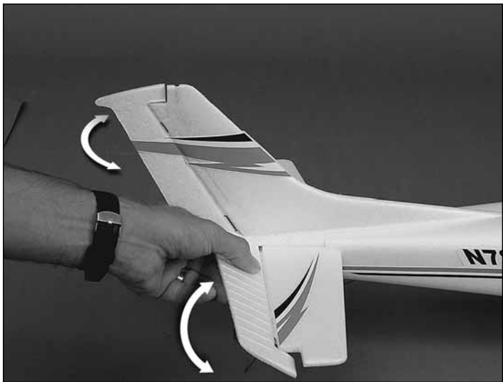
❑ 6. Move the rudder back-and-forth and the elevator up-and-down to make certain everything is operating smoothly. If there is much resistance or if something doesn't seem right, remove the fin and stab from the fuselage and make sure you have the pushrods hooked up correctly. Then reinstall and try again.
