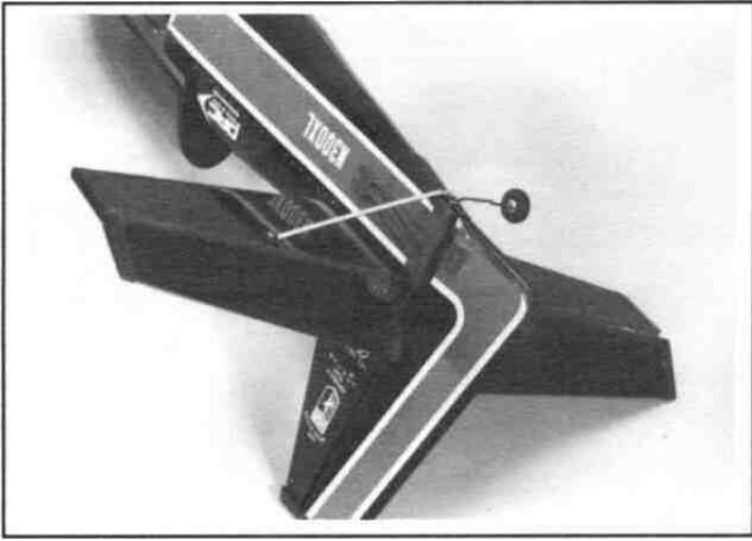
4 Drill six 3mm holes for the three horns. Make sure that you drill straight through to the other side
