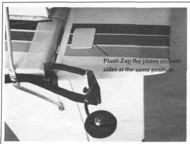
(1) Glue (use PlastiZap) the rectangular mounting plates to the rudder so that they are centered, one on each side, over the tail control arm that is "inside" the rudder.
