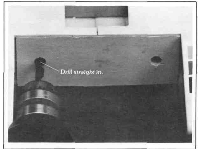
(9) Drill two 8mm holes into the wing joiners for the dowel rods.
