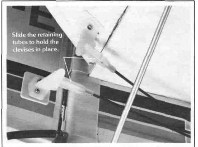
(9) Attach the respective control rods to each horn. Use the middle hole of the horn. Turn on the radio system and adjust the clevises for centered control surfaces
