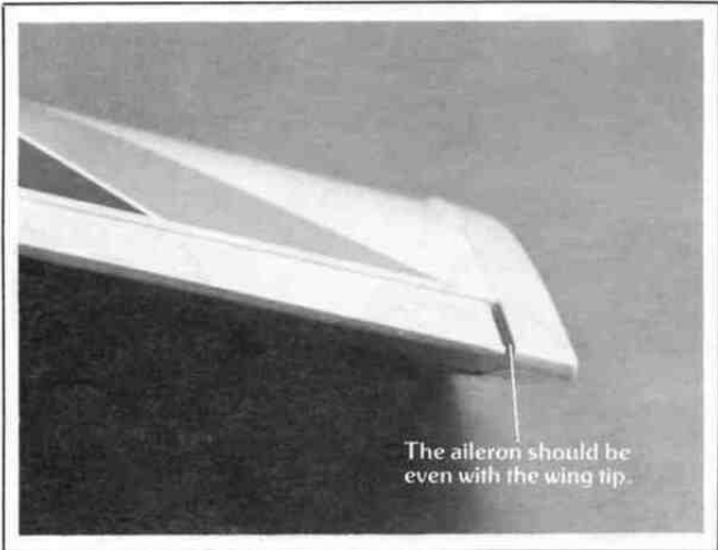
(8) Connect the aileron servo to the receiver and check the movement of the ailerons. Make sure that both ailerons are neutral when the servo is neutral. Adjust the clevises as needed.
