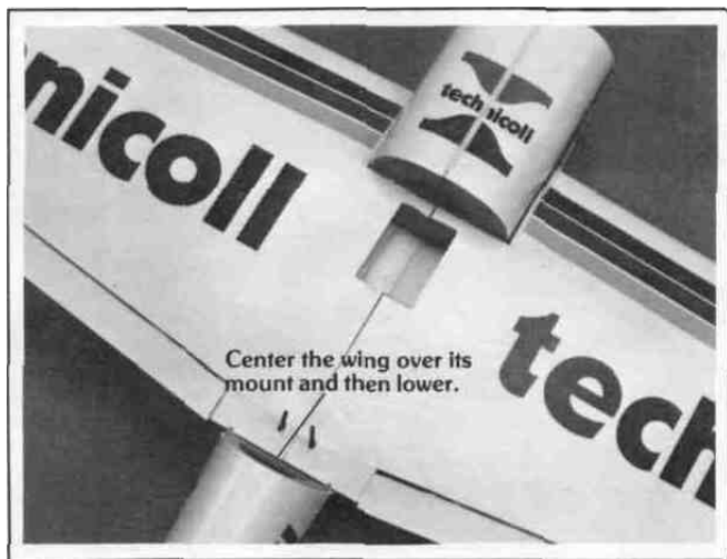
(16) After the epoxy has cured, place the wing into the fuselage as shown. Put the front in first, aligning the dowel rods in the holes. Once in place, lower the back into position.
