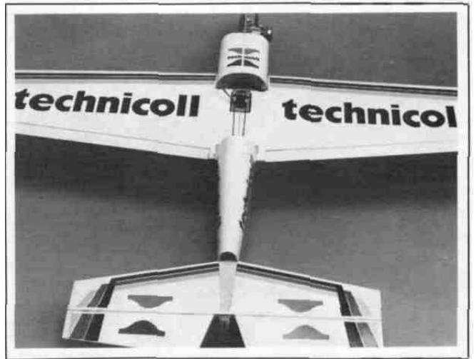
(5) Next, remove the stabilizer and apply epoxy to the wedge. Reinstall the stabilizer and re-center like before.
