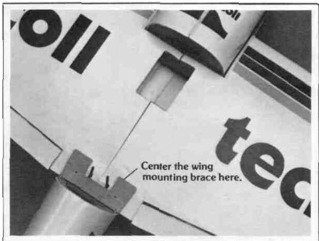
(17) Place the wing mounting brace onto the wing as shown and center the wing and brace with the fuselage. NOTE The two indentations on the brace should face up. PlastiZap it on.
