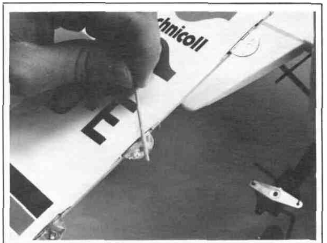
(18) Place a small amount of epoxy on the hinges, in the groove and on the end of the tail control arm. (It is a good idea to place some petroleum jelly onto the hinge center joint (point of movement) to keep out any epoxy.)
