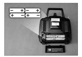
To install the batteries, slide the battery door down. Insert the cells as shown in the diagram, making sure to note proper polarity for each cell. Close the battery door.
