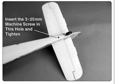
$\hfill 3$  3. Secure the horizontal stabilizer to the fuselage with a 3  $\times$  25mm machine screw.
