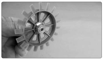
□ 1. Insert the collet prop adapter through the engine louvers.
