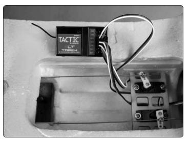
2. Plug the throttle into channel-3 on the Tactic receiver.
