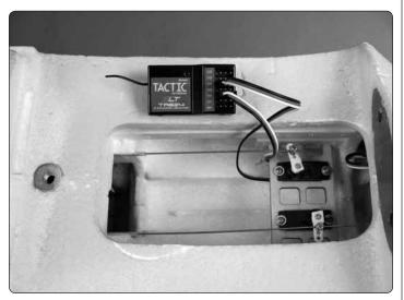
$\hfill\square$  1. Plug the elevator servo into channel-2 on the Tactic receiver. Plug the rudder servo into channel-4 on the Tactic receiver.
