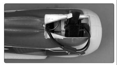
□ 5. With the transmitter still switched on, connect the LiPo motor battery to the electronic speed control. The motor will produce a low tone. Moving the right stick on the transmitter up and down will move the elevator on the plane up and down. If the motor does not beep and the elevator does not move, the receiver will need to be bound to the transmitter.
