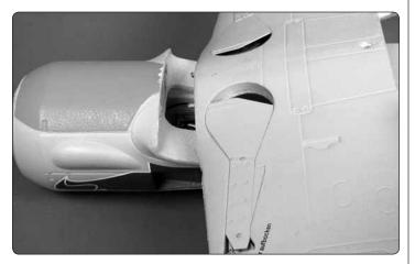
□ 2. Insert the two wing dowels in the leading edge of the wing into the two holes at the front of the wing saddle.
