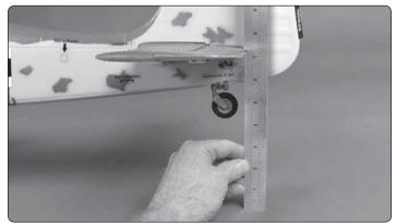
□ 3. Still without the propeller mounted on the motor, switch on your transmitter and connect the motor battery. Place a ruler next to the trailing edge of the elevator at the widest part (from front-to-back).
