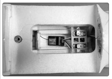
□ 3. Peel the backing from one side of the double-sided tape. Attach it to the back of the receiver. Peel the backing from the other side of the double-sided tape and attach it to the bottom of the servo compartment.
