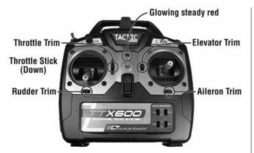
□ 3. Position the throttle stick (left stick) to idle (all the way down) and switch on the transmitter. The power indicator light should be glowing a steady red. A flashing red light and an audible tone indicates low voltage. If this happens, replace the batteries before connecting the flight battery.
