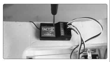
□ 6. To bind the receiver to the transmitter, remove the receiver from the plane. Make sure the throttle stick is down in the idle
