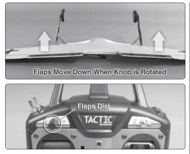
□ 8 . Operate the flaps from the transmitter. On the Tactic TTX600 the flaps are operated using the dial. Check that the flaps move down the same amount and do not bind in the up position. If one of the flaps moves down more than the other or binds in the up position, loosen the screw in the screw lock pushrod connector and adjust the pushrod until the flaps operate correctly. Check that all the screws in the screw lock pushrod connectors are tight against the pushrods.
