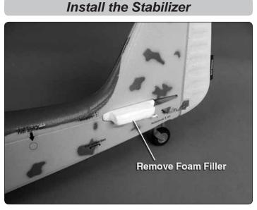
□ 1. Remove the foam filler piece from the horizontal stabilizer opening.
