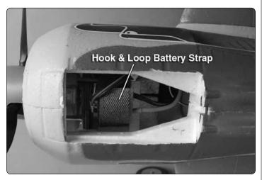
□ 1. Insert the motor battery in the fuselage and secure it with the hook and loop strap, but do not connect it to the ESC.
