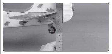
□ 4. Use the transmitter to move the elevator up and measure the distance it moved from center. This is your "up" control throw. Measure the down elevator control throw following the same procedure. Compare the up and down elevator throw to the recommended elevator throw below. Measure and compare the rudder and aileron throws as well.
