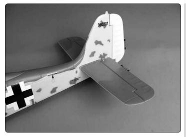
2. Carefully insert the horizontal stabilizer in the fuselage.
