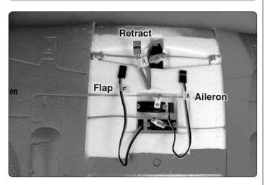
Before mounting the wing, we have found it is helpful to label the servo wires for the ailerons, flaps and retracts. This takes the guesswork out of reconnecting the servo wires to the receiver. We use a small piece of masking tape on each wire and label the ailerons 'A', the flaps 'F, and the retracts 'R'.
