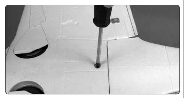
$\Box$  4. Secure the wing to the fuselage with a 6×25mm nylon wing bolt.
