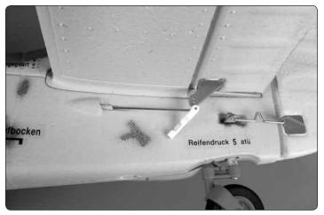
2. Unclip the Faslink from the elevator pushrod.
