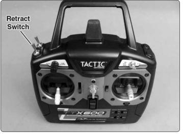
□ 6. Operate the retracts from the transmitter. On the Tactic TTX600 the retracts are operated from the forward switch. Check that the retracts lock in the down position and do not bind in the up position. If one of the retracts does not lock down or binds when retracted, loosen the screw in the screw lock pushrod connector and adjust the pushrod until the retract operates correctly. Check that all the screws in the screw lock pushrod connectors are tight against the pushrods.
