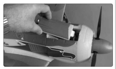
2. Install the battery hatch.
