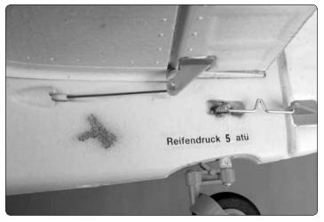
□ 3. Insert the pushrod in the outer hole of the elevator control horn.
