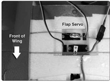
$\Box$  7. On the Tactic TTX600 the flaps plug into channel 6.
