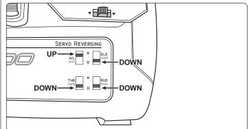
□ 2. Check that the servo reversing switches are configured as shown.
