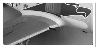
□ 4. Insert the two guns in the holes in the wing. Check that the guns do not interfere with the retracts.
