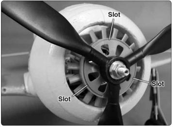
□ 2. Install the collet prop adapter on the motor shaft. Slide the propeller on the prop adapter and secure it with the prop washer and prop nut. Align the propeller so that the slots in the engine louver are between the propeller blades. Then, tighten the prop nut with a wrench.
