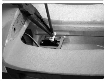
□ 1. Remove the  $2.5 \times 5$  mm machine screw in the screw lock connector on the elevator servo. Center the elevator and apply a small drop of threadlocker to the threads of the screw. Hold the screw lock connector with a needle nose pliers and reinstall the screw in the screw lock connector, tightening it against the elevator pushrod. Move the elevator stick, checking that the elevator moves in the correct direction.
