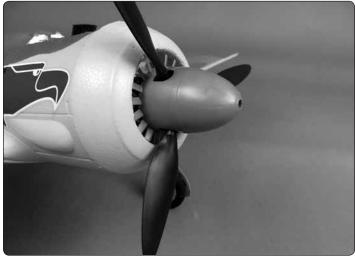
$\Box$  3. Position the spinner back plate over the propeller. Then, secure the spinner cone and back plate to the prop adapter with a  $3 \times 25$  mm machine screw.
