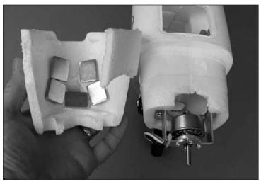
□ 4. Now that you can see the fuselage and the wires from the ESC, continue cutting and peeling the rest of the cowl off. Note that the cowl may have weight attached to the inside to balance the plane. This weight may need to be removed and attached to the new cowl to balance the plane at the correct CG.
