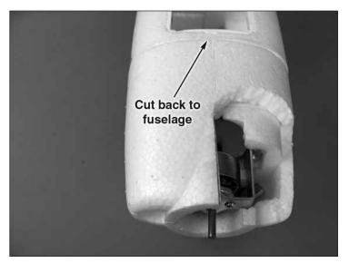
□ 2. Carefully peel off one side of the cowl to expose the fuselage. Use a sharp hobby knife to finish the top cut back to the fuselage. Do not cut into the fuselage under the cowl.
