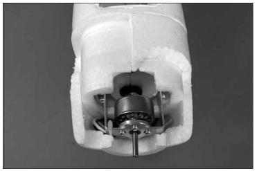
□ 3. Work your fingers under the top of the cowl and carefully peel the cowl off the fuselage.
