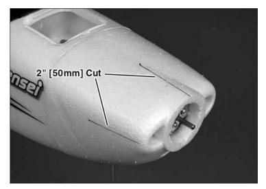
□ 1. Make three cuts, one on the top and one on each side, 2" (50mm) long.
