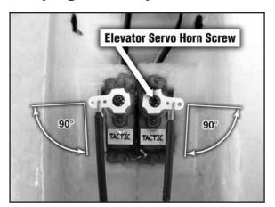
In order to complete step 4, it may be necessary to remove the elevator servo horn. When step 4 is complete, re-install the servo horn in the pre-removal position on the elevator servo shown on page 6 of the manual.
