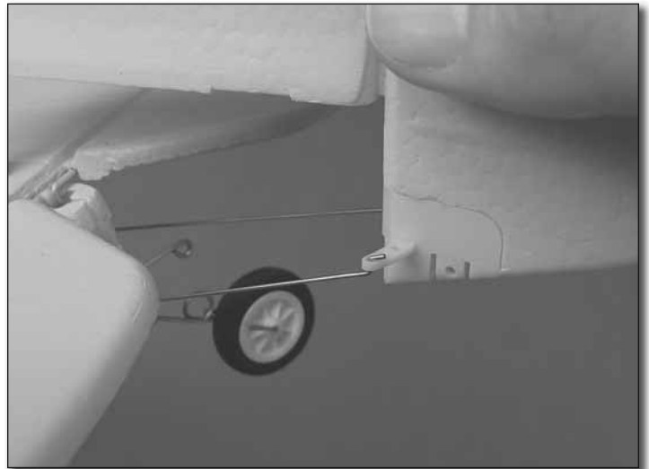
❑ 5. Same as the elevator pushrod, guide the two rudder pushrods partway up through the guide tubes in the fuselage. Connect the pushrods to the outer holes in the rudder horn, then rotate the rudder 90° to lock the pushrods in.
