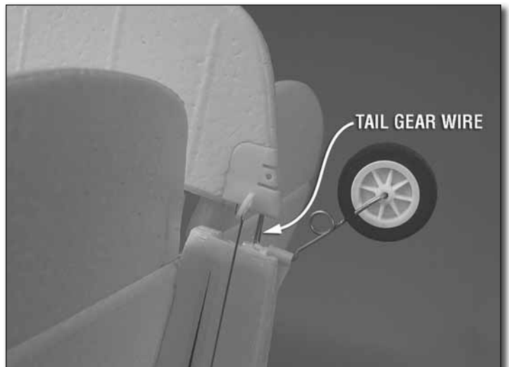
❑ 6. Prepare to join the vertical stabilizer assembly to the fuselage by inserting the tail gear wire partway into the rudder.
