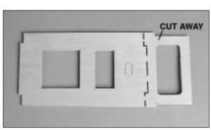
□ 1. Locate the plywood **servo tray.** Cut off the portion of the tray indicated by the dashed line.
