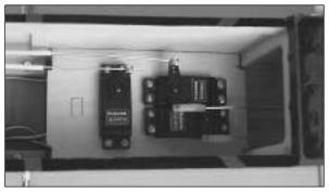
□ 10. Turn on the transmitter and receiver. Set the throttle to full open. Install the pushrod into the other screw-lock pushrod connector, then open the carburetor on your engine to full open. Connect the throttle linkage following the same steps as used for the nose gear steering.
