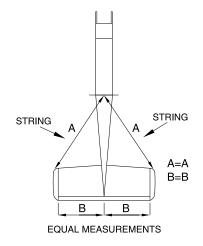
□ 7. Attach one end of monofilament string or a small tape measure to the T-pin. Measure back to the end of the stabilizer on the left side of the fuselage. Do the same for the right side of the fuselage. When the distance from the T-pin to each side of the stabilizer is equal, the stab is properly positioned.
