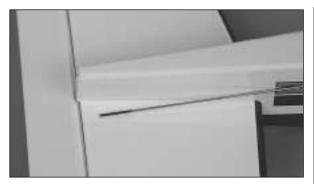
□ 2. Insert the threaded end of the elevator pushrod into the fuselage, working it around until the end of the rod is extending through the exit hole on the lower left side of the fuselage.
