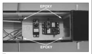
□ 3. Use 6-minute epoxy to glue the tray in place inside of the fuselage. When properly installed, the servo tray will rest firmly on the rear former.
