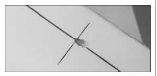
□ 3. At the intersection of the two lines drill a 1/8" [3mm] hole in the fuselage bottom. The hole needs
