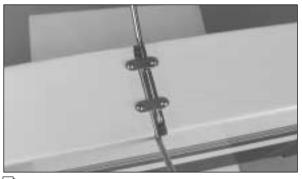
□ 1. Insert the **landing gear struts** into the holes in the bottom of the fuselage. Secure the landing gear with the two metal straps. Mount them in place with **3mm x 10mm self-tapping screws.**
