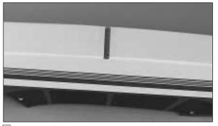
□ 2. Turn the fuselage over and cut away the covering on the bottom of the fuselage for the landing gear.
