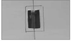
□ 5. Locate the plywood **aileron servo tray.** Place it in position over the opening in the bottom of the wing. With a felt-tip pen, mark the position of the servo tray.
