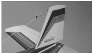
☐ 17. After cutting the servo arms, thread the antenna through the hole you drilled in the fuselage and attach the antenna to the vertical fin with a rubber band and T-pin as shown above.
