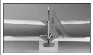
□ 13. After the epoxy has cured on the stabilizer, test fit the **fin** into the slot in the top of the fuselage.
