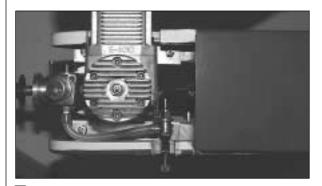
□ 2. Put your engine onto the **engine mount**. **Note:** Depending on your engine you may need to cut away portions of the fuselage sides for clearance for the muffler or needle valve. Place the engine mounting straps over the mounting rails of the engine. Screw the mounting rails in place with the **4mm x 15mm screws** and **4mm lock washers**.
