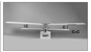
☐ 11. With the stabilizer in place in the rear of the fuselage, step back a few feet and look at the stabilizer in relation to the wing. The distance from the top of the stab to the bottom of the wing should be the same. If each end of the stabilizer is not equal in distance from the wing, lightly sand one side of the opening until both ends of the stabilizer measure the same distance from the wing.
