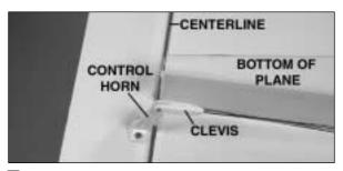
□ 5. Position the elevator control horn on the elevator following the same procedure used for the rudder.
