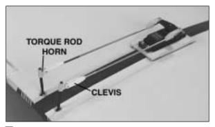
□ 12. Install the clevises on the threaded ends of the pushrods by turning the clevis 14 times. Thread the nylon torque rod horn onto the aileron torque rod and then attach the clevis to the horn.
