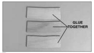
□ 1. Locate three plywood wing joiners. Using 6-minute epoxy, glue them together to form the wing joiner.
