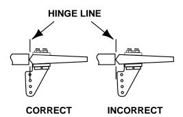
□ 4. Position the **rudder control horn** on the rudder. Make a mark with a felt-tip pen where the holes need to be drilled. **Note:** When installing the control horns, the centerline of the control horn holes must be the same as the center line of the hinge joint as shown in the above sketch. Drill a 1/16" [1.5mm] hole through the marks you just made. Insert the **2mm x 20mm** screws through the control horn backplate.
