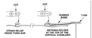
□ 15. Cut off two leftover servo arms as shown in the above diagram. These will be used to make a simple strain relief for your receiver antenna.
