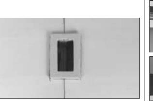
□ 7. Use 6-minute epoxy to glue the servo tray to the opening in the bottom of the wing. **Important Note:** Before gluing the tray in place, test fit your servo into the wing. The opening is deep enough to accommodate most servos. If it is not deep enough for your particular brand of servos, glue the servo tray to the two 1/4" [6mm] balsa blocks included in the kit and then, glue the blocks to the wing with epoxy.
