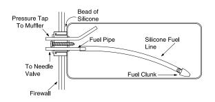
▲ 4. Assemble the fuel tank using the above sketch and the following instructions. Push the two **aluminum tubes** through the **rubber stopper** until 1/2" [13mm] of the tubes protrudes from the front of the stopper. Slide the **large cap** onto the front of the stopper and the **small cap** onto the back. Insert the **stopper screw** into the center hole in the front of the cap, then just begin to screw it through the stopper into the aft of the stopper cap.
