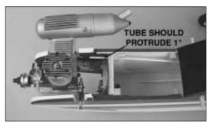
□ 3. Remove the **fuel tank compartment cover** from the fuselage. Locate the **white nylon tube** and cut it to a length of 9". Install it through the predrilled hole in the firewall. Epoxy the tube in place so that 1" of the tube protrudes through the firewall.
