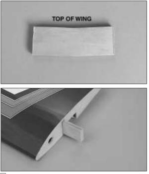
□ 2. After the glue has cured, test fit the joiner into the **wing.** Be sure that the upward angle of the joiner is towards the top of the wing.
