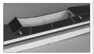
□ 4. Using 6-minute epoxy, glue the two **wooden dowels** in place at the wing saddle.
