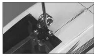
□ 6. Slide the 18" wire **control rod** into the white nylon tube. Install the wire onto the control horn and retain it in place with the **1/16**" wheel collar and **4-40 set screw.**
