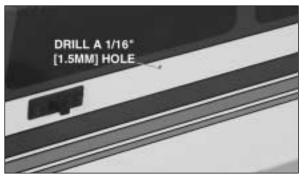
16. Drill a 1/16" [1.5mm] hole in the fuselage.
