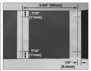
■ 8. Put masking tape onto the fuel tank compartment cover as shown. Mark lines on the tape at the dimensions shown in the photograph. Drill four 1/16" [1.5mm] holes at the intersection of the lines, drilling through the cover and the four hardwood blocks in the fuselage. Secure the hatch to the fuselage with four 2.6mm x 12mm screws.
