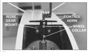
↓ 4. Install the nose gear control horn parallel to the nose gear axle and tighten the mounting screw against the flat side of the wire. Next install a 4mm x 10mm collar on top of the control horn and secure with a 3mm x 4mm screw. Slide the nose gear shaft through the nose gear mount. Secure the gear in place with another 4mm x 10mm collar and a 3mm x 4mm screw.
