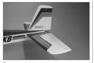
☐ 7. Set the rudder and elevator so they are in the neutral position as shown.
