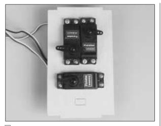
■ 2. Using the hardware that comes with your servos, install the servos as shown. Use a 1/6" [1.5mm] drill to pre-drill the holes for the servo mounting screws. If you do not pre-drill the holes there is a chance that the plywood may split.
