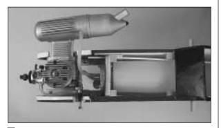
☐ 7. Install the tank into the fuel tank compartment. Apply a bead of silicone sealant around the fuel tank cap when installing the tank into the fuselage. Attach silicone fuel line from the tank to the carburetor and muffler pressure fitting.
