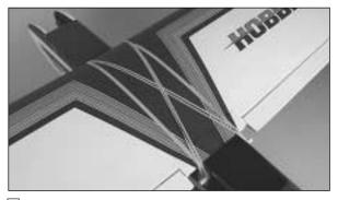
10. Use a few rubber bands and mount the wing in place on the wing saddle.
