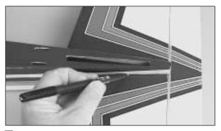
■ 8. Once the stab has been properly positioned, use a felt-tip marker and trace the outline of the fuse onto the stabilizer. Do this on both the top and bottom of the stabilizer.
