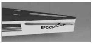
□ 12. Once you have the stabilizer properly fit to the fuselage, remove it and apply 6-minute epoxy to the stabilizer where you cut the material away and to the wing saddle. Slide the stabilizer into the fuselage. Re-check to be sure the stabilizer is positioned properly and that it is in the correct position in relation to the wing.
