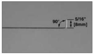
□ 5. Locate one of the 18" wire **control rods.** Make a 90° bend 5/16" [8mm] from the end of the wire.
