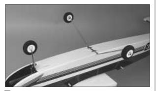
□ 7. Install the **wheel** on the nose gear. The nose wheel has a slightly smaller axle hole than the remaining two wheels. Install a 4mm x 10mm wheel collar and secure it with a 3mm x 4mm screw. Install a **5mm x 10mm wheel collar** on each side of the main landing gear. Then install the wheels and the other 5mm x 10mm wheel collar. Secure the wheel collars with the 3mm x 4mm screws. All three wheels should turn freely. If not, trim the inside of the wheel slightly.
