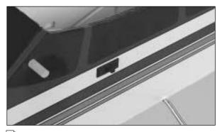
↓ 4. On both sides of the fuselage there is a cut out for your radio switch. Cut away the material on one side of the fuselage for the switch harness.
