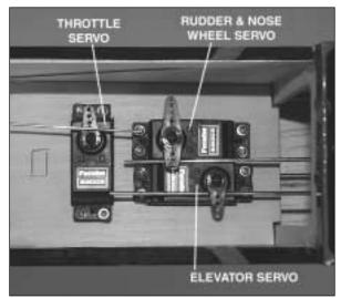
□ 6. Center the trims on the transmitter, turn on the transmitter and receiver and allow the servos to center themselves. Once they are centered, install the servo arms onto the servos, positioning the arms as shown in the photograph.
