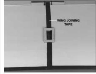
■ 8. Locate the blue **wing joining material.** Peel off the backing and carefully place it over the seam on the top and bottom of the wing.
