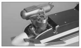
□ 18. Install the propeller recommended by the engine manufacturer along with the spinner.
