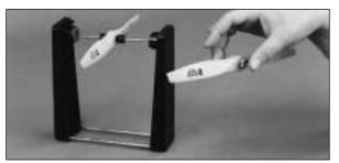
We use a Top Flite Precision Magnetic Prop Balancer<sup>™</sup> (TOPQ5700) in the workshop and keep a Great Planes Fingertip Balancer (GPMQ5000) in our flight box.
