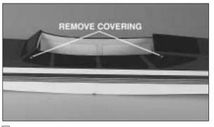
□ 3. Cut away the covering at the wing saddle for the wing hold down dowel holes.
