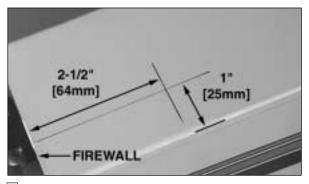
□ 2. Draw two lines at the front of the fuselage with a felt-tip pen. Draw the lines using the dimensions shown in the above photograph.
