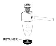
□ 9. Locate a screw-lock pushrod connector, a 4-40 set screw and the nylon retainer. Install it on the remaining arm on the rudder servo by first sliding the nose gear steering pushrod through the hole in the fitting and then assembling the screwlock pushrod connector as shown in the above sketch. Set the nose wheel to be straight and then tighten the 4-40 set screw onto the pushrod wire.
