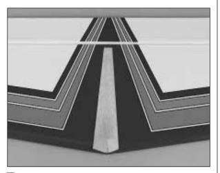
□ 9. Cut away the covering inside of the lines you made on the stab. Do this on both the top and the bottom of the stabilizer, being careful not to cut into the wood sheeting.
