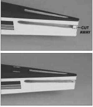
□ 1. Cut away the covering at the rear of the **fuselage** for the horizontal stab, fin and pushrod openings. Cut away the remainder of the stab opening at the rear of the fuselage with your hobby knife.
