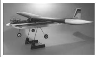
L 1. The balance point (C.G.) is located 3-1/2 [89mm] back from the leading edge of the wing. Balance your Hobbistar 60 using a Great Planes C.G. Machine<sup>™</sup> Airplane Balancer (GPMR2400) for the most accurate results. This is the balance point at which your model should balance for your first flights. Do not at any time balance your model outside the recommended range.
