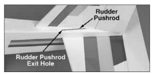
□ 13. Locate and pierce the covering from the rudder pushrod exit hole on the top of the fuselage, left of the fin. **Note:** An easy method to locate the exit hole under the covering is to insert the wire pushrod into the outer pushrod tube just behind the rudder servo and note where the pushrod wire comes out under the covering.
