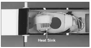
□ 1. Make a strap, the same way you made the battery strap. Route the strap through the front hole in the battery tray and back through the middle hole. Position the **electronic speed control** (ESC) on the battery tray and secure it with the strap, leaving the metal heat sink exposed. Trim off the excess strap.
