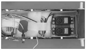
□ 6. Make a fourth strap, the same way you made the two battery straps. Route the strap through the back hole in the battery tray and back through the middle hole. Plug the two servos and the electronic speed control into the receiver. Wrap the receiver in foam rubber and position it on the battery tray, securing it with the strap. Trim off the excess strap.
