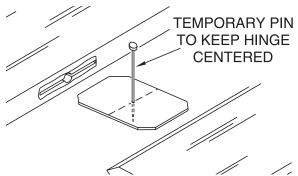
□ □ 5 Test fit the ailerons to the wing with the hinges. If the hinges don't remain centered, stick a pin through the middle of the hinge to hold it in position.
