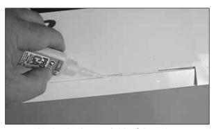
□ 7. Apply six drops of thin CA to the top and bottom of each hinge, waiting a few seconds between drops to allow the CA to soak in. Do not use CA accelerator. After the CA has fully hardened, test the hinges by pulling on the aileron.
