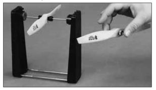
Carefully balance your propeller before you fly. An unbalanced prop can be the single most significant cause of vibration that can damage your model. Not only will mounting screws and bolts loosen, possibly with disastrous effect, but vibration may also damage your radio receiver and electronic speed control.
