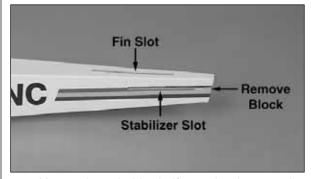
□ 1. Use a sharp hobby knife to trim the covering from the slots for the stabilizer and fin at the aft end of the **fuselage**. You can feel the slots for the stabilizer on both sides of the fuselage. The slot is located close to the red stripe. Also cut the wood block from the aft end of the slots. The slot for the fin is in the top of the fuselage.
