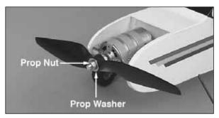
□ 2. Slide the **propeller** onto the prop adapter. The front of the prop has 9 x 5.5 lettering molded into it. Secure the propeller to the prop adapter with the aluminum **prop washer** and **prop nut**. Hold the prop adapter retainer while tightening the prop nut. Make sure the prop is securely attached to the motor shaft.
