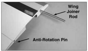
$\square$  9. Insert the 7/32" x 6-7/8" [5.5mm x 174.6mm] steel wing joiner rod in the forward hole in the wing root rib of the left wing half. Insert the 3/32" x 1" [2.3mm x 25.4mm] anti-rotation pin in the aft hole in the wing root rib.
