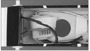
□ 2. Connect the red and black wires from the motor to the red and black wires from the electronic speed control. Make sure the wires are securely connected. If any of the metal connector is visible, wrap it in electrical tape to prevent the wires from shorting and damaging the electronic speed control.
