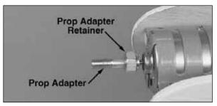
☐ 1. Slide the aluminum **prop adapter** over the motor shaft. Slide the aluminum **prop adapter retainer** over the prop adapter. **Note:** The hole through the prop adapter retainer is beveled. The side with the larger hole goes on first.
