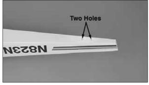
□ 3. Use a sharp hobby knife to trim the covering from the two holes on the bottom aft end of the fuselage.
