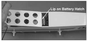
□ 4. Insert the lip on the **battery hatch** under the sheeting at the aft end of the battery compartment. Lock the battery hatch in position by rotating the battery hatch retainer over the battery hatch.
