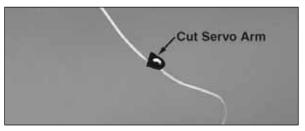
☐ 18. Make a strain relief by trimming the servo arm you cut off previously, so that only two holes remain. Thread the receiver antenna through the first hole and back through the second hole. Position the strain relief so that it is approximately 6" [152.4mm] from the receiver. The strain relief will hit the side of the fuselage, preventing the receiver antenna from being pulled loose from the receiver.
