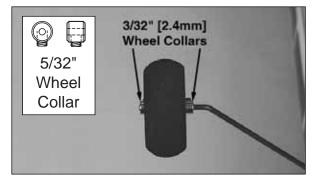
□ 5. Slide a 3/32" [2.4mm] wheel collar on one of the landing gear wires, followed by a wheel and a second wheel collar. Secure the wheel collars to the landing gear wires with 4-40 set screws. Repeat the process for the second landing gear wire. Make sure the wheels rotate freely.
