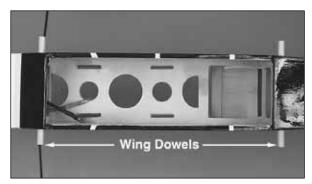
□ 2. Insert and center the 1/4" x 4" [6.4mm x 101mm] wing dowels in the holes in the fuselage.
