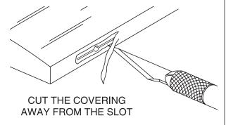
□ □ 3. Use a sharp #11 blade to cut a strip of covering from the hinge slots in the wing and aileron.
