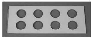
□ 1. The **battery hatch cover** has holes cut in the plywood. Use a hobby knife with a sharp blade to trim the covering from over the holes.
