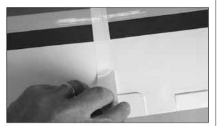
□ 11. On the top and bottom of the wing, apply the 1" [25.4mm] wide **wing joiner tape**, centering on the joint between the two wing halves.
