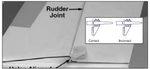
☐ 14. From the aft end of the model, reinsert the pushrod wire with the control horn on it into the rudder outer pushrod tube. Guide the end of the pushrod through the screw-lock pushrod connector on the rudder servo. Position the control horn on the leading edge of the rudder so that the pushrod holes are aligned with the joint between the rudder and fin. If it is not aligned properly with the joint, the plane will turn better one way than the other.
