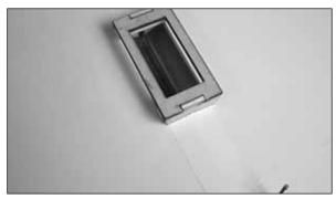
☐ 12. Glue the aileron servo tray onto the tabs in the servo opening.
