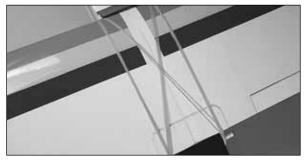
□ 2. Again place a rubberband around the aft wing hold-down dowel and stretch it over the top of the wing, this time crossing over to the other side of the fuselage before placing it around the forward wing hold-down dowel.
