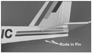
□ 5. Insert the fin in the fin slot. The two threaded rods go through the two holes in the stabilizer and out the two holes in the bottom of the fuselage.
