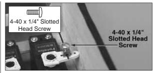
☐ 16. With the transmitter and electronic speed control switched on, set the rudder to neutral (straight with the fin). Secure the rudder pushrod in the screw-lock pushrod connector with a 4-40 x 1/4" slotted head screw. Cut off the excess pushrod.
