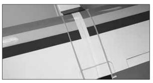
☐ 1. Center the wing on the fuselage. Place a rubberband around the aft wing hold-down dowel and stretch it over the top of the wing, placing it around the forward wing hold-down dowel. Attach a second rubberband on the other side of the fuselage.
