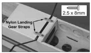
□ 4. Secure the main landing gear wires to the fuselage with two nylon landing gear straps and four 2.5mm x 8mm sheet metal screws. Note: The pilot holes are predrilled under the covering and the covering only needs to be pierced.
