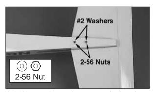
□ 6. Place a **#2 washer** over each fin rod and secure the fin to the fuselage with **#2-56 nuts**. Do not overtighten the nuts and crush the wood. The nuts should be just tight enough to prevent the stabilizer from moving side to side.
