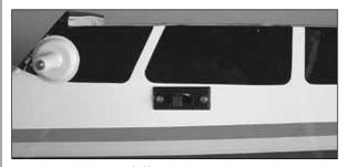
□ 3. Install the on/off switch in the opening under the second window on the left side of the fuselage.
