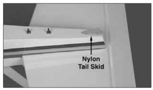
□ 2. Insert the nylon **tail skid** in the holes. If the tail skid fits loosely, a drop of glue in each hole will secure the tail skid.
