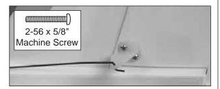
□ 15. Mark the two control horn mounting hole locations. Move the control horn out of the way and drill a 3/32" [2.4mm] hole through the rudder, at both hole locations. Insert two 2-56 x 5/8" machine screws through the control horn and the rudder. Install the control horn back plate on the other side of the rudder.
