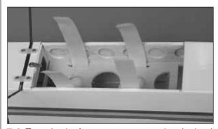
□ 3. To make the **battery straps**, overlap the hook and loop material by approximately 2" [50.8mm]. Insert the battery straps, from the inside the fuselage, through the slot in one side of the battery tray and back out the slot on the other side of the battery tray. Install a front and back battery strap.
