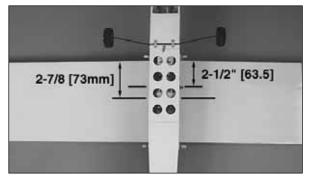
□ 1. Use a felt-tip pen or 1/8"-wide tape to accurately mark the C.G. range on the bottom of the wing on both sides of the fuselage. The C.G. range is located between 2-1/2" [63.5mm] and 2-7/8" [73mm] back from the leading edge of the wing.
