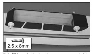
□ 3. Slide a plastic dowel cap over one end of the wing dowel. Secure the **dowel cap** with a 2.5mm x 8mm sheet metal screw. Install the other three dowel caps and secure them with 2.5mm x 8mm sheet metal screws.
