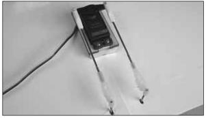
☐ 17. Install the wire into the hole in the servo arm using a nylon FasLink as shown in the sketch.
