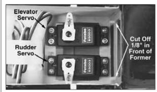
□ 10. Install the servo arms on the rudder and elevator servos so that they are perpendicular to the centerline of the servo. Also use a hobby knife to trim the outer pushrod tubes approximately 1/8" [3.2mm] in front of the former.
