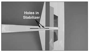
□ 4. Insert the stabilizer and center it in the stabilizer slot. The side with the red, yellow and blue stripe faces upward. The two holes through the stabilizer should be aligned with the fin slot in the top of the fuselage.
