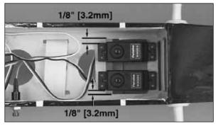
□ 4. Follow the instructions that came with your radio system to properly install the rubber grommets and metal eyelets on your servos. Place two servos in the servo tray as shown. Position them so that they are approximately 1/8" [3.2mm] from the side of the servo tray.
