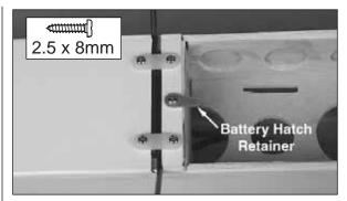
□ 2. Use a 2.5mm x 8mm sheet metal screw to attach the aluminum **battery hatch retainer** to the fuselage at the front of the battery hatch. Note that the pilot hole for the screw has been drilled under the covering and the covering only needs to be pierced. Tighten the screw completely, then back it off 1/8 of a turn. The hatch retainer should require some pressure to rotate it. If it is too loose, it may rotate during flight, allowing the battery hatch to come off.
