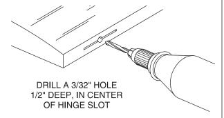
□ □ 2. Drill a 3/32" hole, 1/2" deep in the center of each hinge slot to allow the CA to "wick" in. Follow-up with a #11 blade to clean out the slots. Hint: If you have one, use a high-speed rotary tool to drill the holes.
