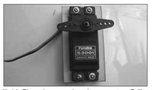
☐ 14. Place the servo into the servo tray. Drill a 1/16" [1.6mm] hole through each of the mounting holes and secure the servo to the tray with the hardware provided with the servo.
