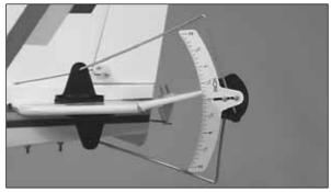
Use a Great Planes AccuThrow (or a ruler) to accurately measure and set the control throw of each control surface as indicated in the chart that follows. If your radio does not have dual rates, we recommend setting the throws at the low rate setting. **NOTE:** The throws are measured at the **widest part** of the elevator and rudder.
