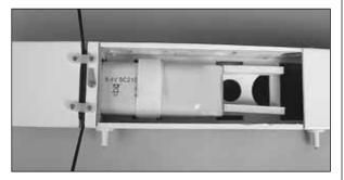
□ 3. Insert the motor battery in the battery compartment. Secure the battery with a hook and loop strap. It is not necessary to plug the motor battery into the electronic speed control until you are ready to fly.
