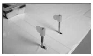
☐ 13. Screw the aileron torque rod horns onto the aileron torque rod wires.
