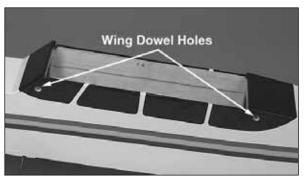
□ 1. Trim the covering from over the wing dowel holes on both sides of the fuselage. The holes are located at the front and back of the wing saddle.
