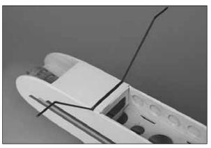
□ 3. Insert the two **main landing gear wires** in the holes, in the slot, at the front of the fuselage.
