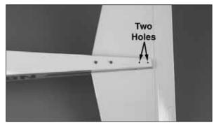
□ 1. On the bottom of the fuselage, at the aft end, are two small holes. Remove the covering from these holes with a hobby knife.
