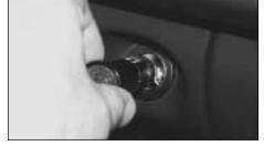
2. Remove the battery pack from the plane. Plug the battery pack into the charger connector. The battery pack will plug in only one way.
