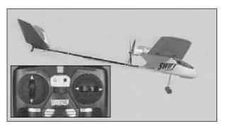
☐ 7. Releasing the left stick will allow your airplane to slowly descend for landing. Fly down wind, beyond your landing spot and turn back into the wind. Release the left stick and the airplane will glide in for a landing.
