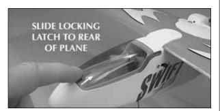
2. After the battery pack is charged, move the canopy locking latch toward the rear of the airplane and lift the canopy.
