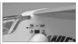
3. Move the ON/OFF switch located on the left side of the fuselage forward to the ON position.
