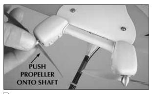
☐ 1. Press the propellers onto the motors. To prevent the props from binding, be sure to leave a small space (about the same thickness of a penny), between the propellers and the back of the motor covers.
