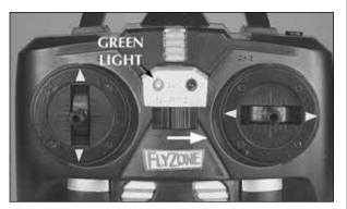
$\square$  1. First switch on the transmitter and make sure the green light is on.
