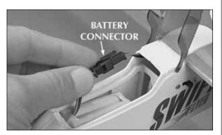
2. Open the canopy on the fuselage and plug the freshly charged battery pack into the plug in the fuselage. The plugs will only go together in the correct direction. Close and lock the canopy.
