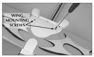
5. Secure the two wing mounting screws, from the small parts bag, into the wing as shown in the above photograph. Do not overtighten them.
